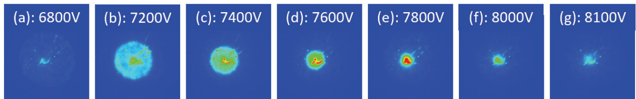
Figure 41: Shape of the scattered beam monitored by the phosphor screen for different einzel voltage: 6800 V (a), 7200 V (b), 7400 V (c), 7600 V (d), 7800 V (e), 8000 V (f) and 8100 V (g). The best focuses occur at 7800 V.
