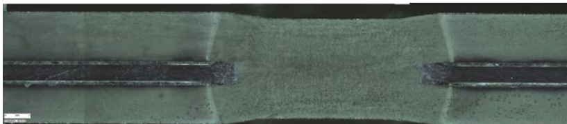
FIGURE D.3 – Point soudé assemblé (stitching)
