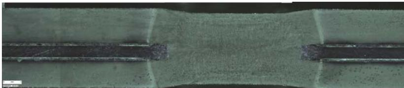
FIGURE D.3 – Point soudé assemblé (stitching)
