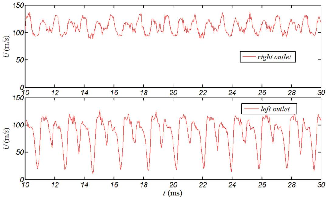
Figure 2-9. Sample velocity evolution pattern in the center of both outlets of Osc.2,  $P_i = 0.20 \text{ MPa}$
