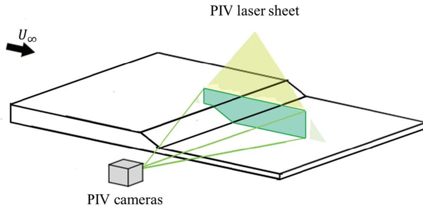
Figure 6-14. Sketch of the PIV system positions
