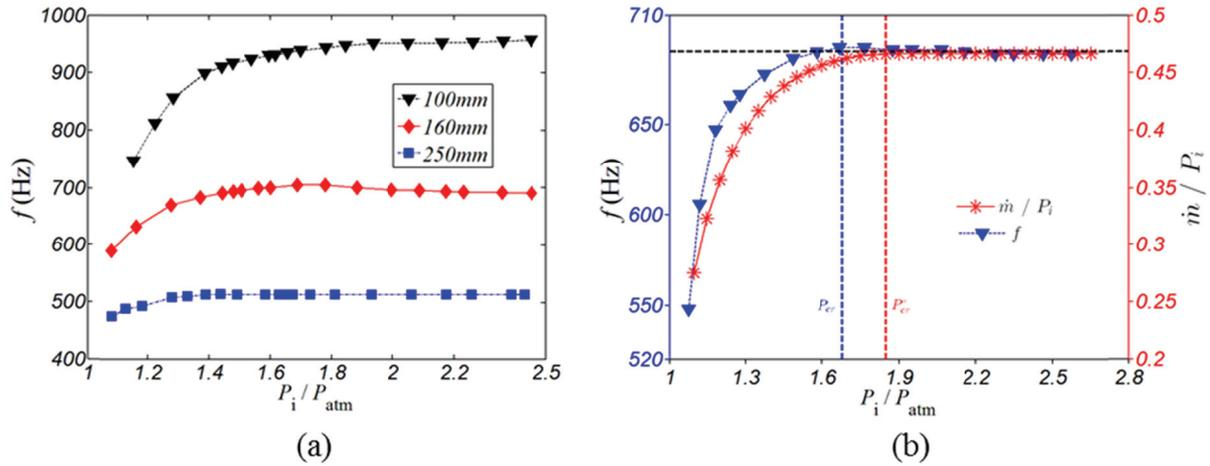
Figure A1-2. a) frequency response vs inlet pressure for different feedback tubes,  $L_t=100, 160, 250$ mm; b) variation of the oscillation frequency and the calculated value of  $\dot{m} / P_i$  with inlet pressure,  $L_t=160$  mm
