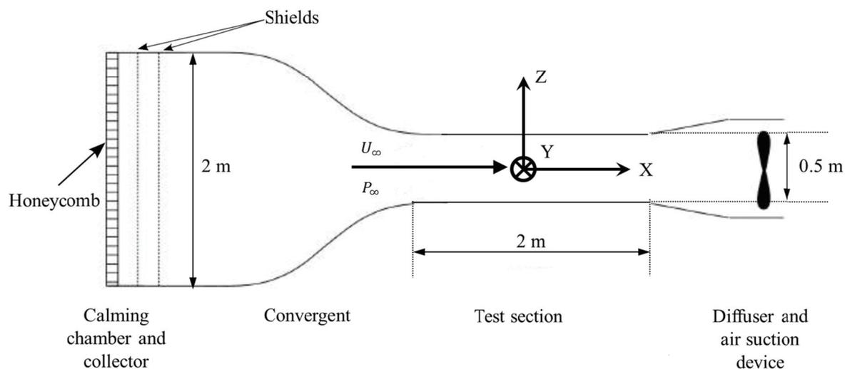
Figure 6-11. Sketch of the wind tunnel S2 in PRISME laboratory
