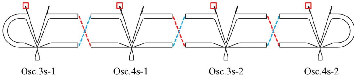
Figure 5-18. Sketch of the configuration used in the numerical simulation of the synchronization of an array of 4 oscillators using the 1<sup>st</sup> proposed inter-connection pattern
