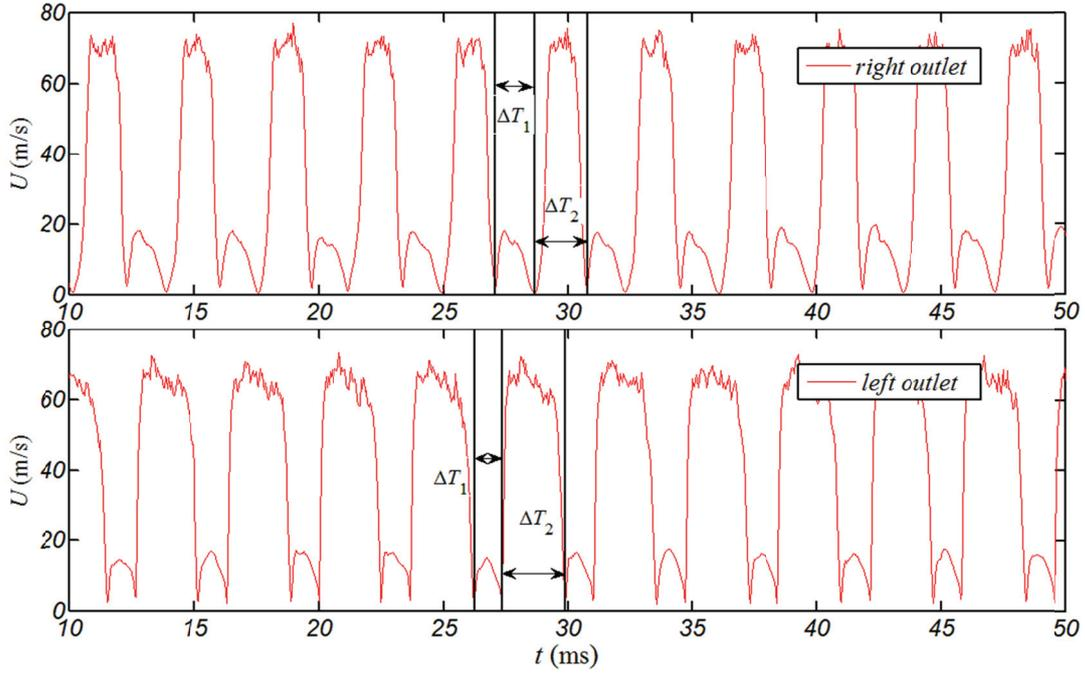
Figure 2-8. Velocity evolution with time in the center of both outlets of Osc.1,  $P_i = 0.20$  MPa
