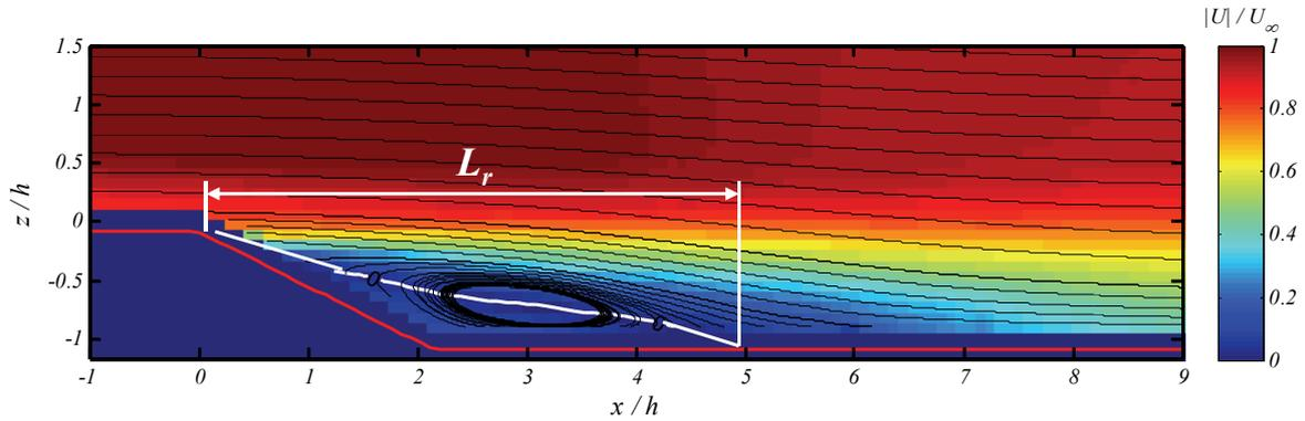
Figure 6-15. Mean flow flow field of the baseline separated flow,  $Re=3.8 \times 10^4$
