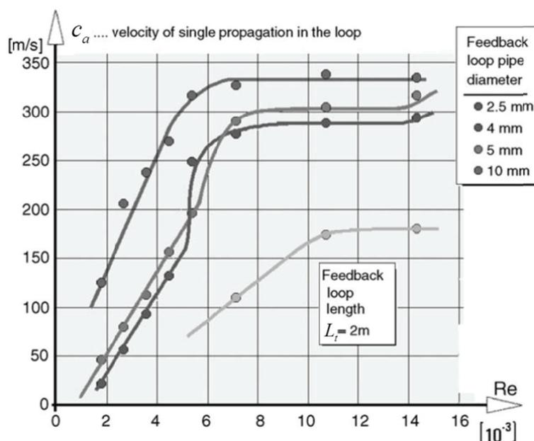
Figure 1-12. Propagation velocity development as a function of inlet  $Re$ , for different feedback tube diameters<sup>31</sup>
