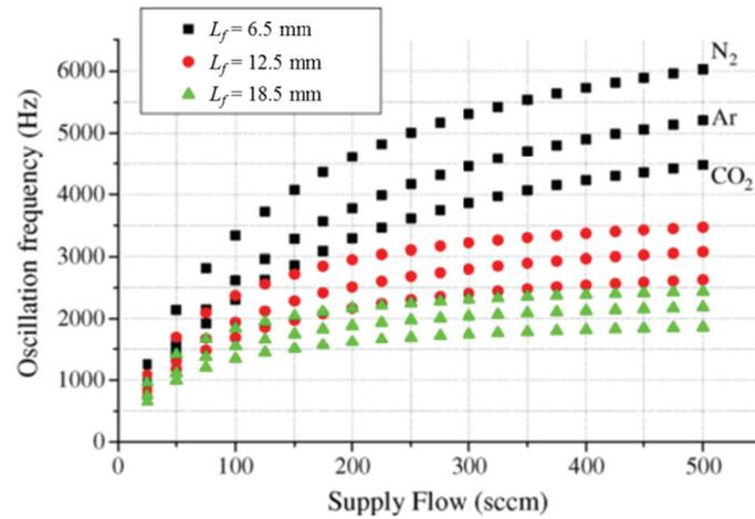
Figure 1-16. Oscillation frequency as a function of FBL  $L_f$ <sup>59</sup>
