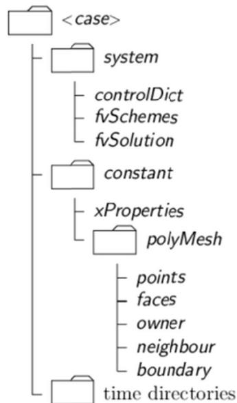
Figure 3-1. Sketch of the organization of an OpenFOAM case folder<sup>79</sup>
