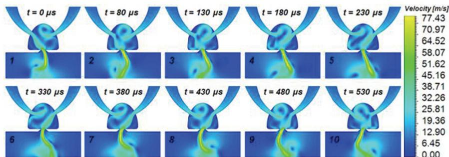
Figure 1-7. Two-dimensional CFD results of a jet-interaction fluidic oscillator internal and external flows<sup>34</sup>
