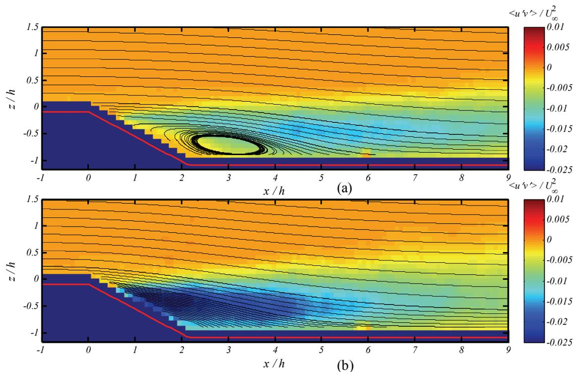
Figure 6-26. Contours of mean flow Reynolds stress component  $\langle u'v' \rangle$ , a) baseline flow; b) controlled flow,  $C_\mu = 0.16\%$
