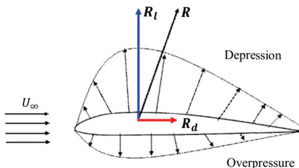
Figure 1-3. Aerodynamic forces on an airfoil section<sup>12</sup>
