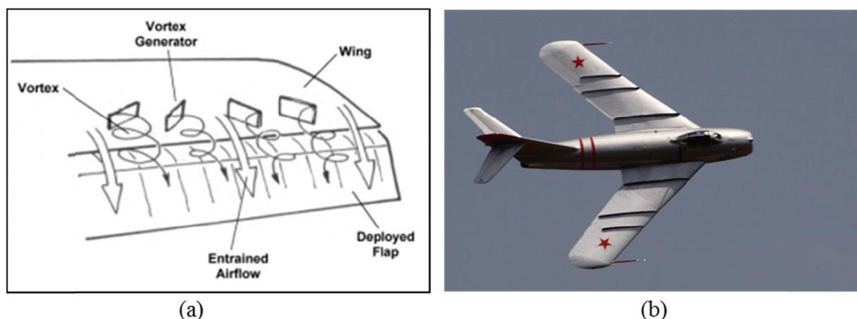
Figure 1-5. a) sketch of a working vortex generator;<sup>15</sup> b) wing fences on the airfoil of Mig-17
