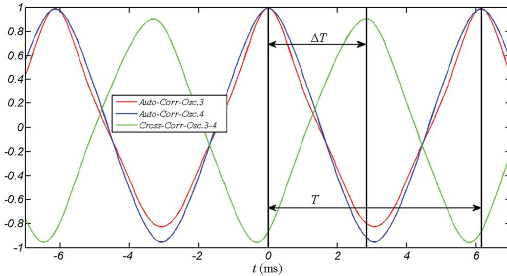
Figure 5-4. Auto-correlation and cross-correlation sequences of the pressure signals from Osc.3 and Osc.4 – 1<sup>st</sup> synchronization method
