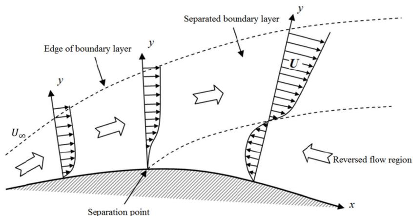
Figure 1-2. Separation of a boundary layer<sup>11</sup>
