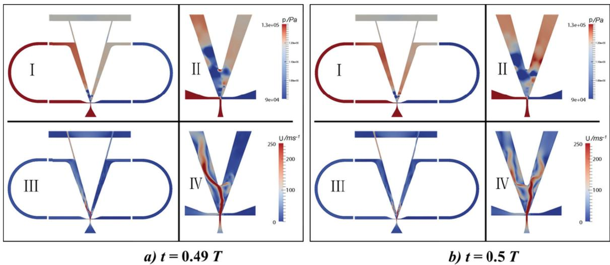
Figure 4-4. Contours of static pressure (upper windows) and velocity magnitude (down windows) in a global view (left windows) and zoomed view (right windows) a)  $t = 0.49 T$ ; b)  $t = 0.5 T$
