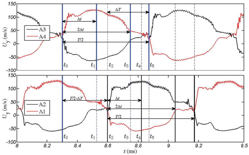
Figure 5-15. Evolution with time of the area-average velocity  $U_y$  in the branch inlet sections A of Osc.3s and Osc.4s, 4<sup>th</sup> method
