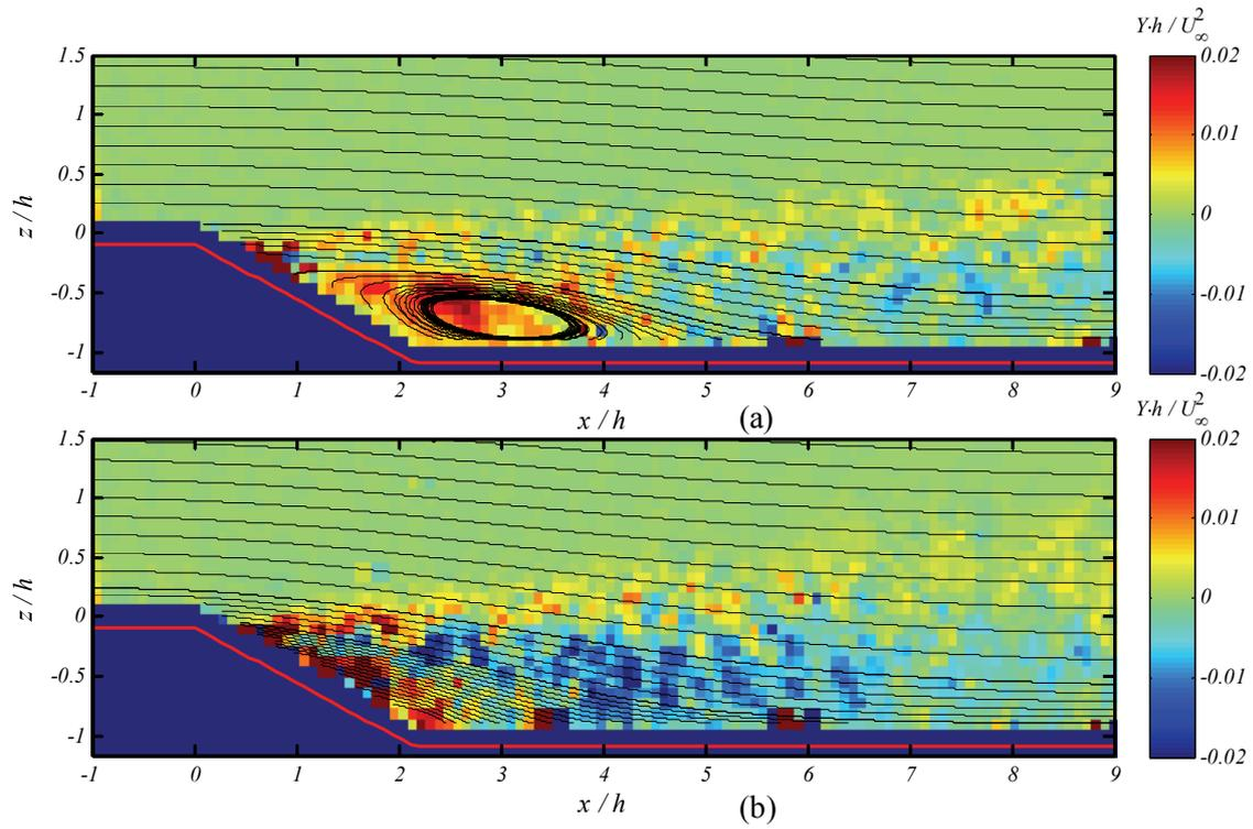
Figure A3- 5. Contours of x direction gradient of Reynold stress component  $\langle u'u' \rangle$ ,  $Y = \frac{\partial \langle u'u' \rangle}{\partial x}$  scaled by  $\frac{U_\infty^2}{h}$ , a) baseline flow; b) controlled flow,  $C_\mu = 0.16\%$
