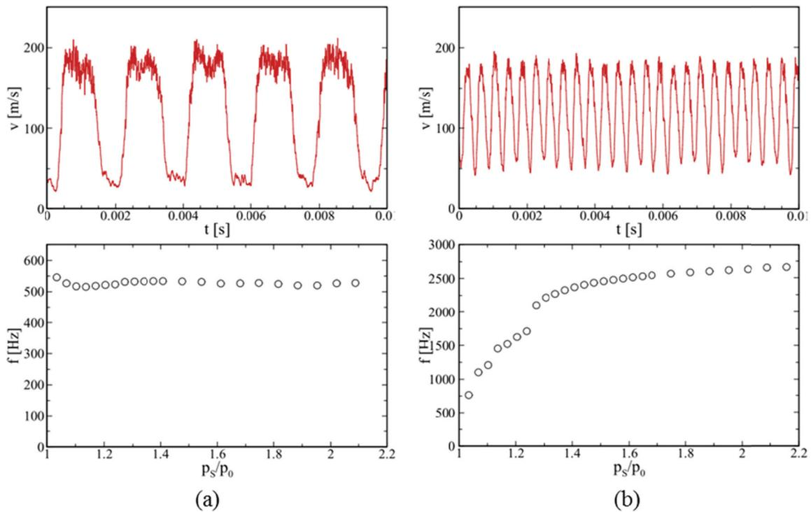
Figure 1-18. Frequency response to inlet pressure and sampled velocity signal by hot wire measurement, a) oscillator A, b) oscillator B<sup>8</sup>
