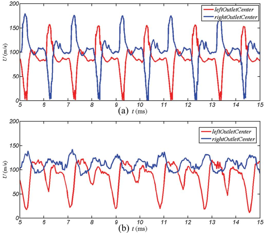
Figure 3-5. Velocity magnitude evolution with time in the center of Osc.2's both left and right outlet slots,  $P_i=0.2$  MPa, a) results from simulation, b) results from hot wire measurements
