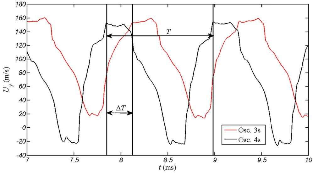
Figure 5-14. Comparison of the velocity  $U_y$  in the center of left outlets of Osc.3s and Osc.4s; 4<sup>th</sup> synchronization method
