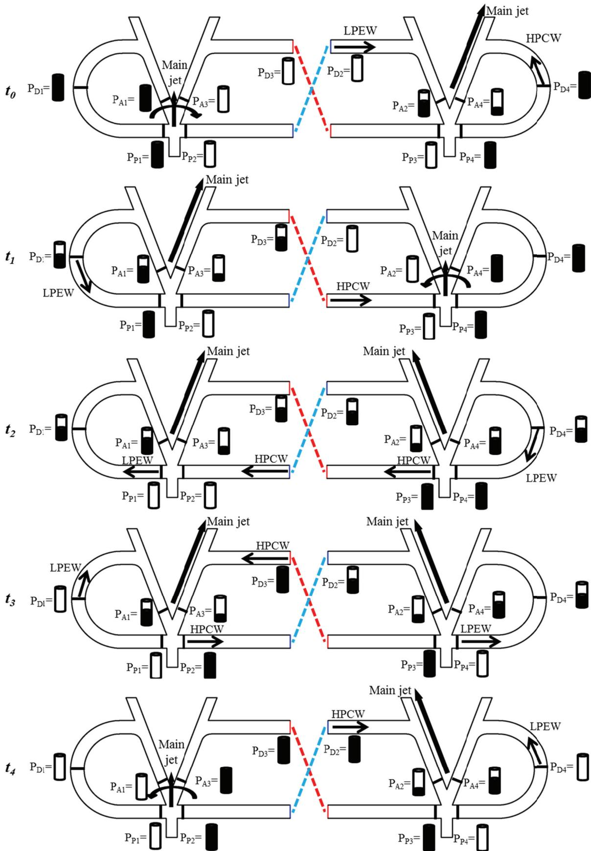
Figure 5-12. Sketch showing the main jets directions and propagation of pressure waves along the feedback loops at each defined critical time; left side Osc.3s, right side Osc.4s
