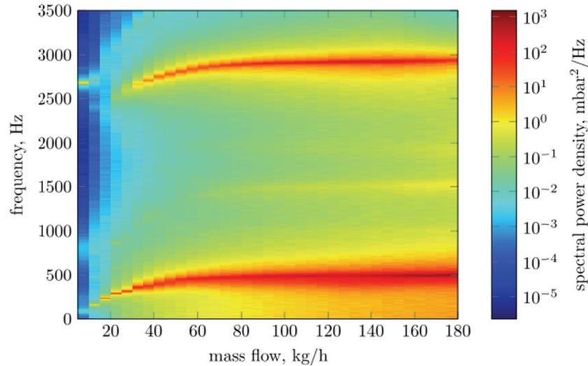
Figure 1-13. Frequency spectra of differential signal between symmetrically paired pressure taps for investigated supply rates<sup>57</sup>
