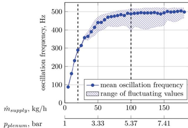
Figure 1-14. Oscillation frequency as a function of the supply rate<sup>57</sup>
