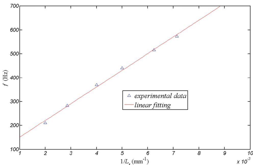
Figure A1-7. Frequency versus inverse value of connection tube length,  $D=3.5$  mm
