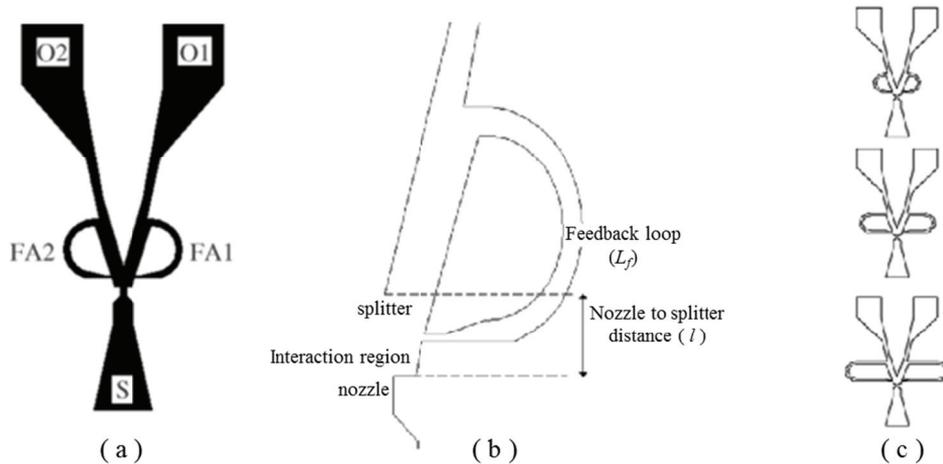
Figure 1-15. Geometrical characteristics of Simoes' device: a) main parts of the device, b) detail of the interaction region, and c) configurations with feedback arms of different lengths<sup>59</sup>
