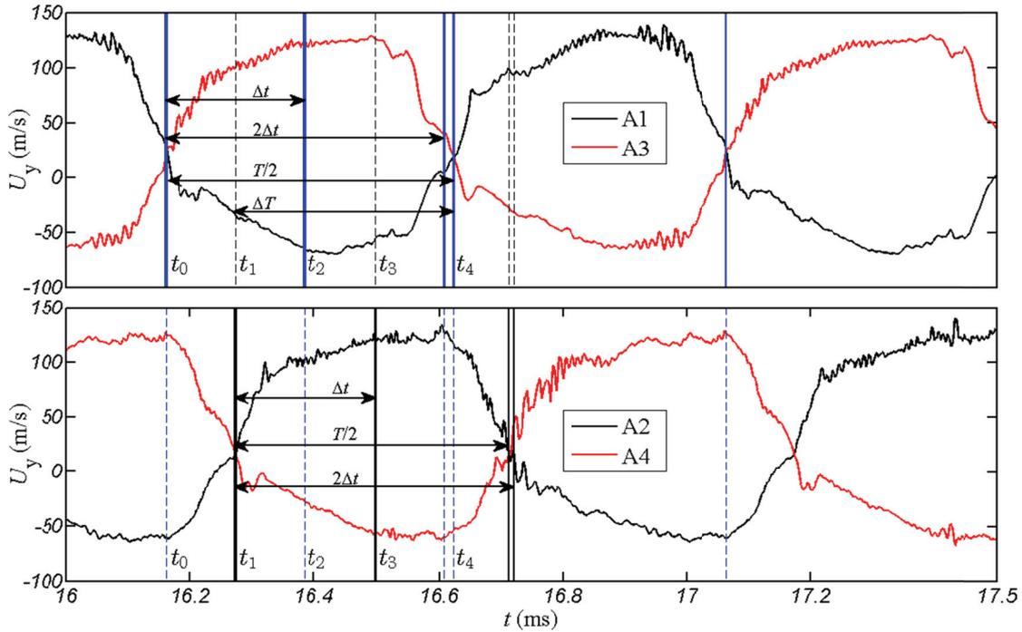
Figure 5-10. Evolution with time of the velocity  $U_y$  in the branch inlet sections A of Osc.3s and Osc.4s
