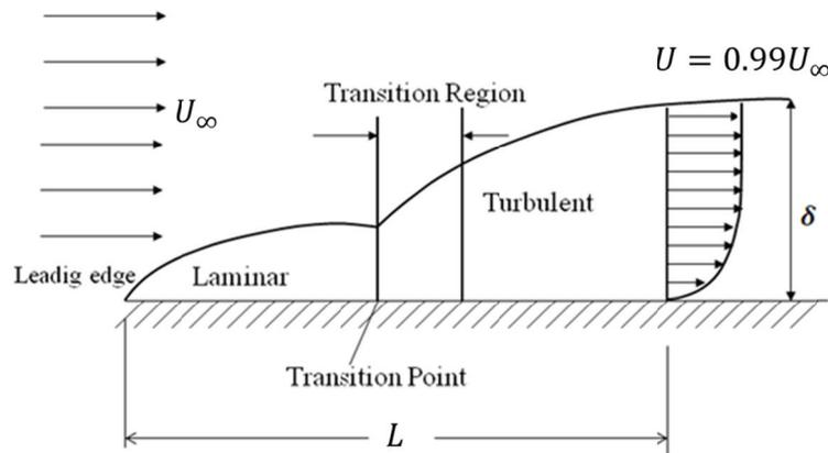
Figure 1-1. Boundary layer on a flat plate
