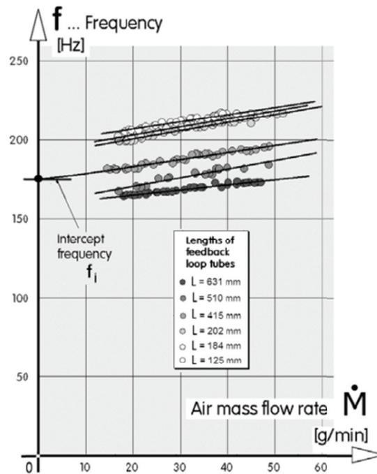
Figure 1-19. Measured oscillation frequency as a function of the inlet flow rate, with different FBLs<sup>64</sup>
