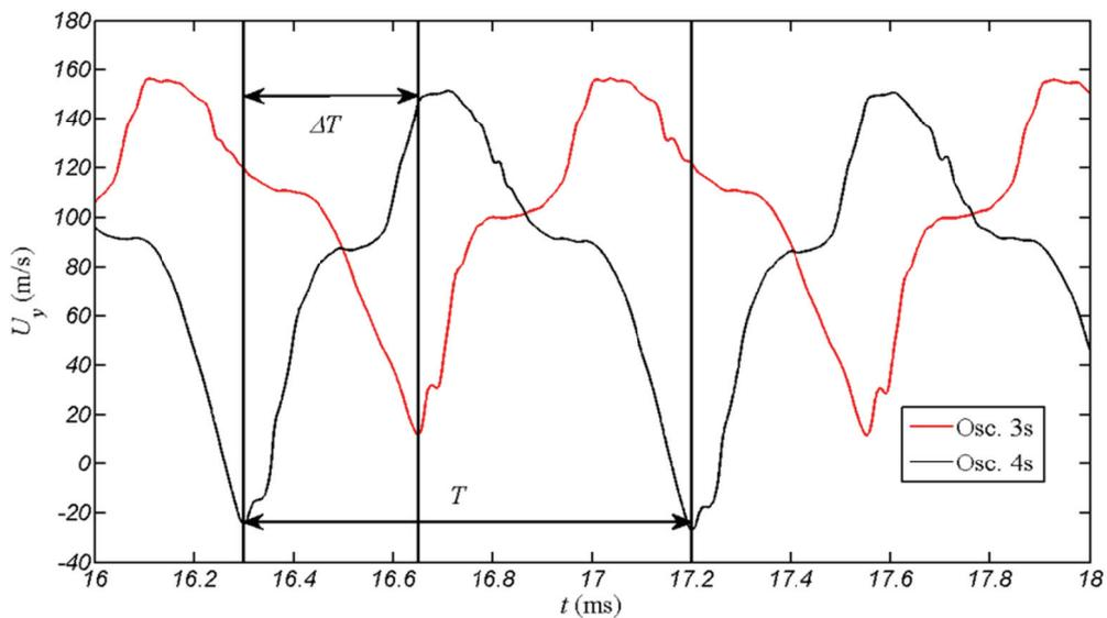
Figure 5-9. Comparison of the velocity  $U_y$  in the center of left outlets of Osc.3s and Osc.4s; 1<sup>st</sup> synchronization method
