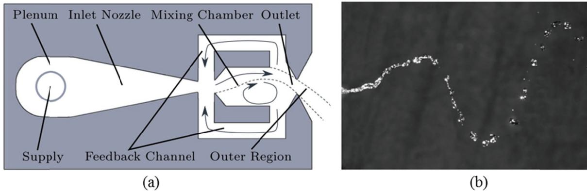
Figure 1-8. a) sketch of the geometry of a sweeping jet Coanda fluidic oscillator and its internal flow pattern; b) its sweeping pattern visualized with water<sup>35</sup>
