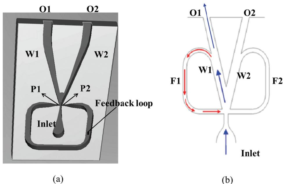
Figure 1-6. Illustration of the basic configurations of wall-attachment fluidic oscillators: (a) sonic oscillator<sup>31</sup> and (b) relaxation oscillator<sup>8</sup>. The primary flow direction is from bottom to top in both cases
