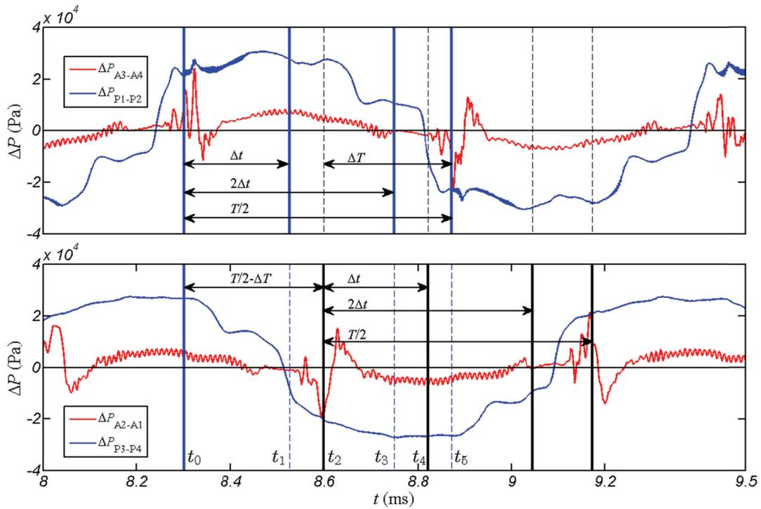
Figure 5-16. Evolution with time of the pressure differences between the control port P and branch inlet A sections of Osc.3s and Osc.4, 4<sup>th</sup> synchronization method
