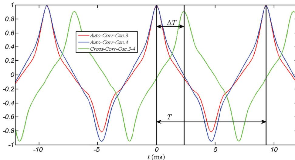
Figure 5-5. Auto-correlation and cross-correlation sequences of the pressure signals from Osc.3 and Osc.4 – 4<sup>th</sup> synchronization method
