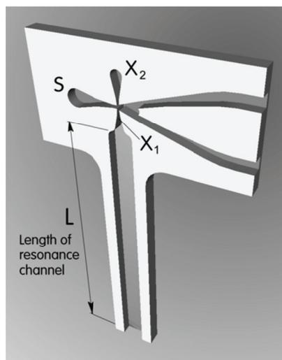
Figure 1-21. New idea of fluidic oscillator proposed by Tesař et al.<sup>65</sup>
