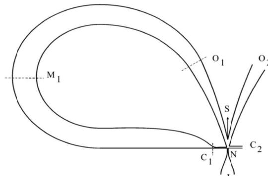
Figure 1-20. Sketch of a mono-stable fluidic oscillator based on an amplifier<sup>58</sup>
