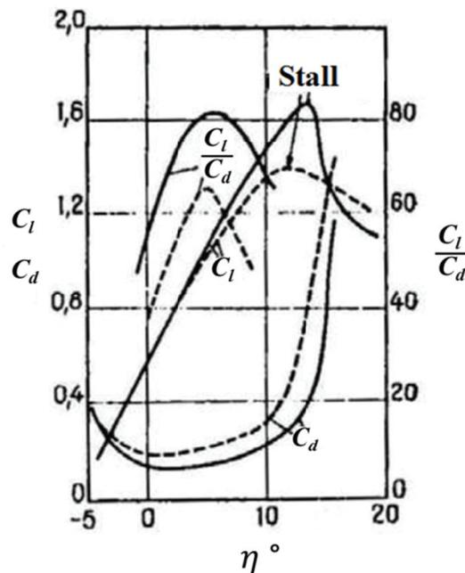
Figure 1-4. Variation of  $C_l$  and  $C_d$  in function of  $\eta$  in case of a plane airfoil.<sup>13</sup> ———  $Re = 6.5 \times 10^5$ ,
