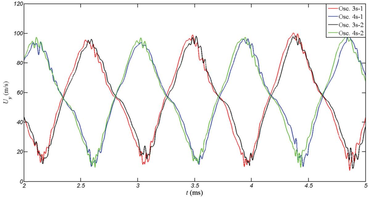
Figure 5-19. Numerical evolution with time of  $U_y$  in the center of the left outlet slot in each oscillator of the array, 4<sup>th</sup> synchronization method
