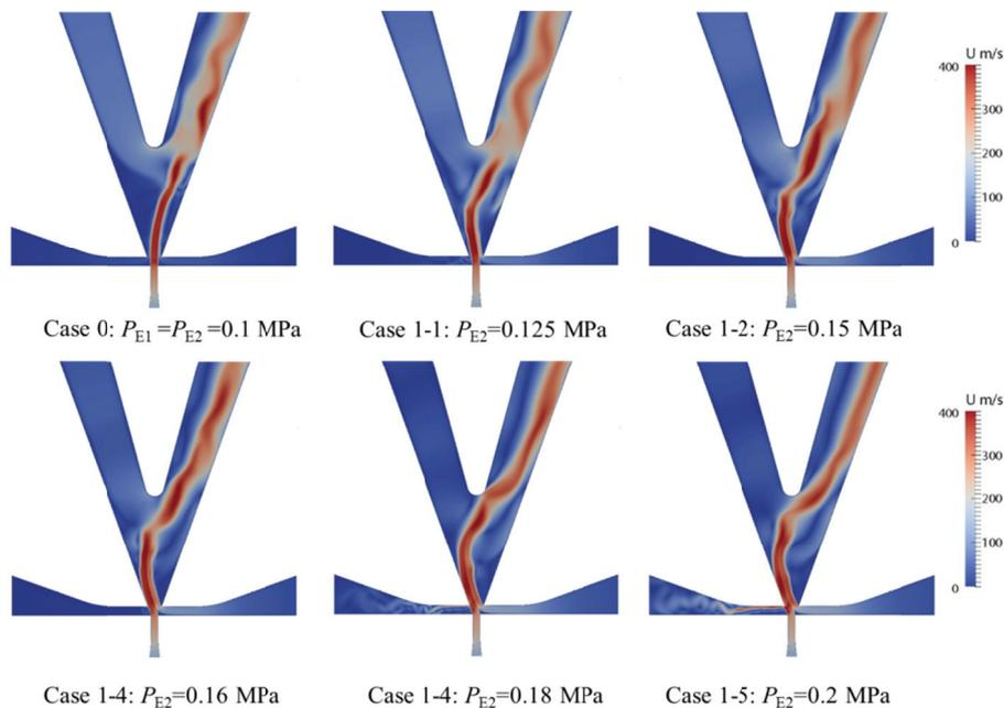
Figure 4-10. Velocity contours in the simplified oscillator model for different values of the pressure  $P_{E2}$  at the right control port.  $P_i = 0.25$  MPa,  $P_{G2} = P_{G1} = 0.1$  MPa,  $P_{E1} = 0.1$  MPa (case 0) or 0.09 MPa for all other cases.
