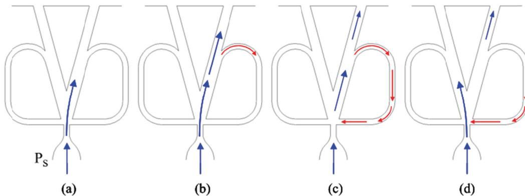
Figure 1-17. Pulsing jet relaxation fluidic oscillator: switching mechanism.  $P_s$  indicates the supply total pressure<sup>8</sup>
