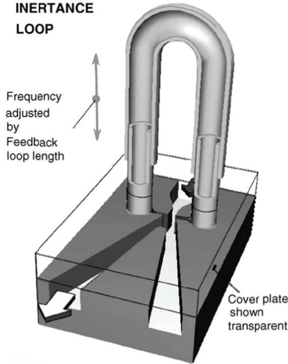
Figure 1-10. A sonic fluidic oscillator based on a bi-stable diverter valve developed by Tesař V. et al. <sup>31</sup>
