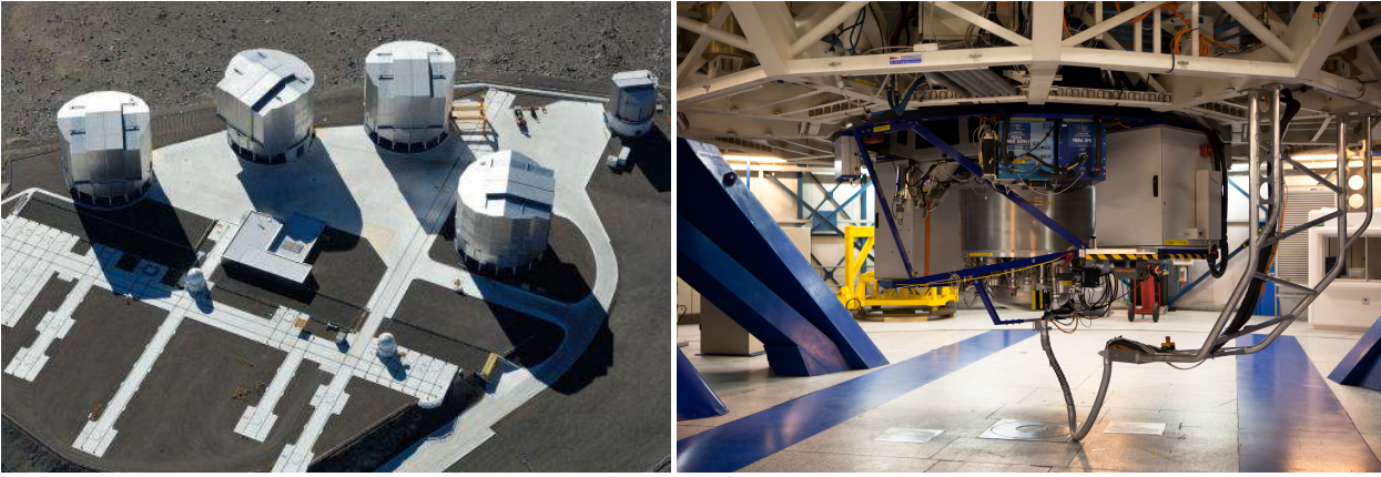
FIGURE 4.8 – Left : The Very Large Telescope’s four 8.2 m Unit Telescopes. Right : The XSHOOTER spectrograph mounted on UT2. Credit : ESO
