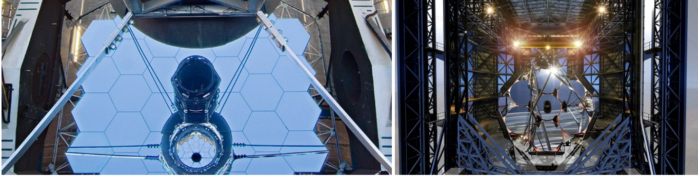
FIGURE 4.10 – Left : Close-up view of the 10.0 m primary mirror of the W.M. Keck telescopes. Credit : WMKO, California Institute of Technology (Caltech). Right : Close-up view of the 6.5 m primary mirror of the Giant Magellan Telescopes. Credit : LCO/GMTO.
