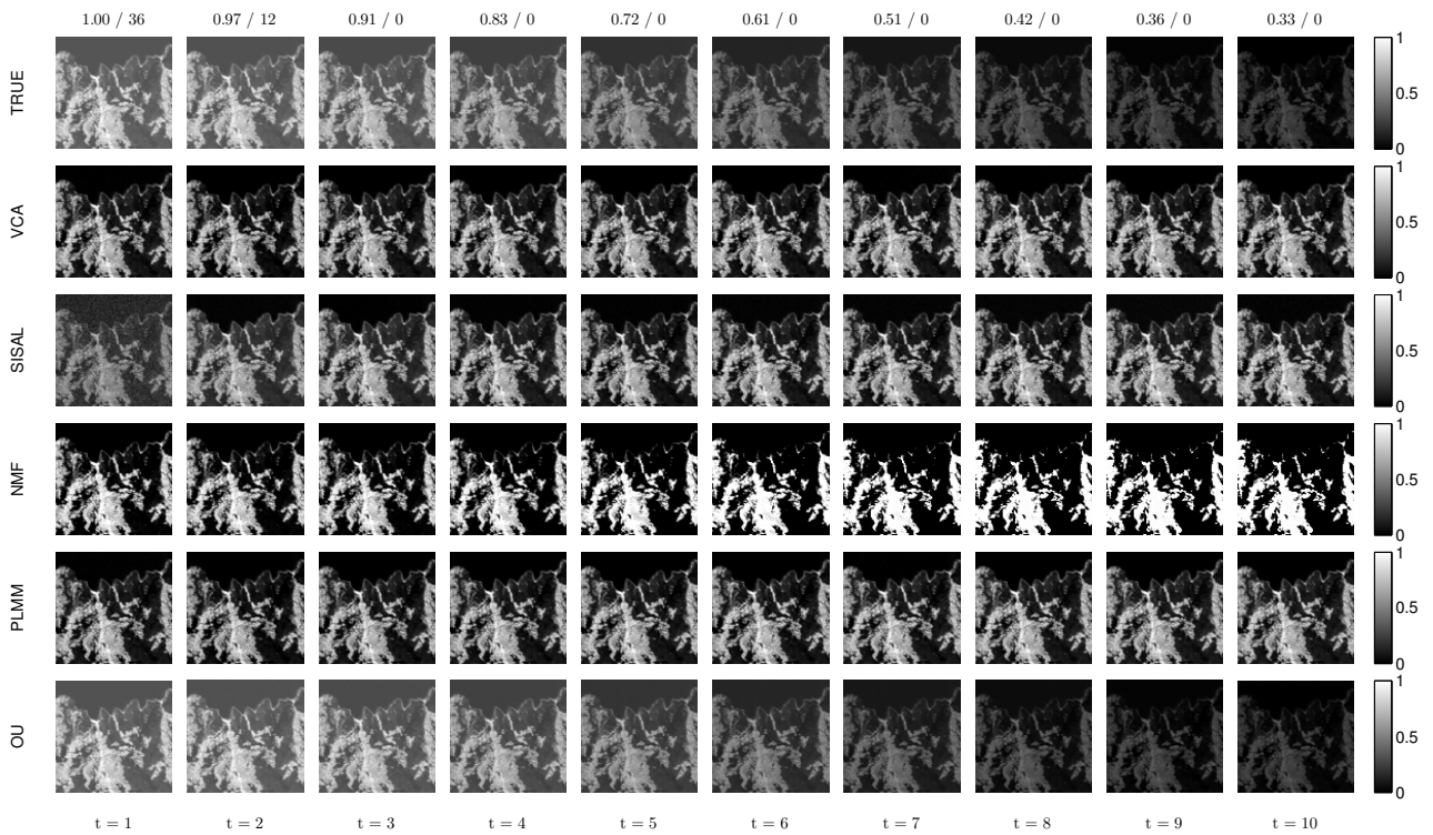
Figure 3.2.: Abundance maps of the first endmember used in the synthetic mixtures. The top line indicates the theoretical maximum abundance value and the true number of pixels whose abundance is greater than 0.95 for each time instant.
