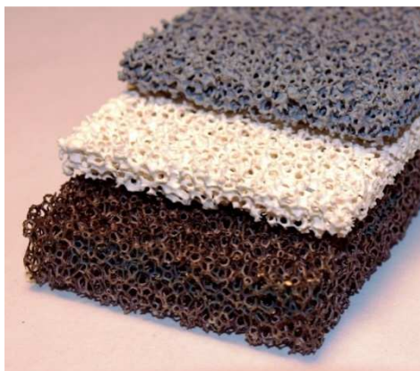
Figure 2.1. A photo of the foam supports used for preparation of structured catalytic systems.
