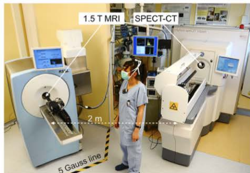
Fig. 1 The two contiguous imaging systems used in this study. No interferences were noticed between the 1.5-T preclinical MRI and the SPECT/CT, set 2 m apart.
