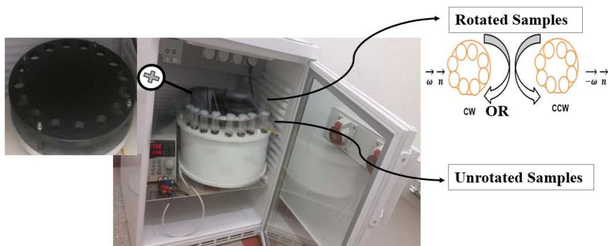
Figure II-18 Experimental setup for crystallization process using rotatory plate inside the fridge.
