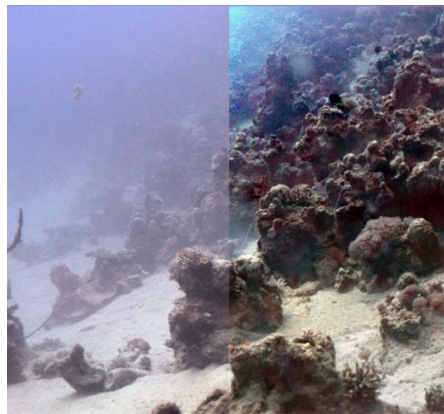
Figure 1.3: An image of the sea bed obtained with a camera. The left side is the raw image, the right side is the processed image. Taken from [47].
