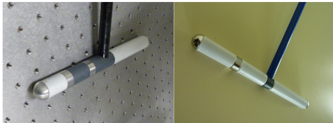
Figure 1.25: The bio-inspired sensor using U-I technology. Left: four macro-electrodes version, right: three macro-electrodes version.
