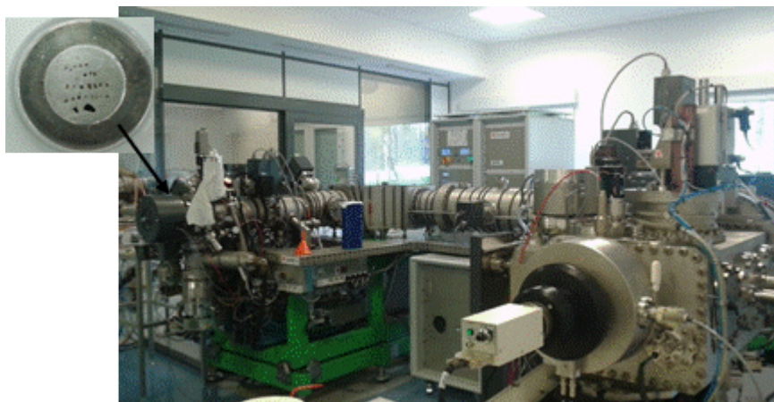
Fig. 3.3 - Cameca IMS 1270 used for SIMS analyses at the CRPG of Nancy. In the left small picture the usual Al-disk fill with indium, prepared for the SIMS analysis.
