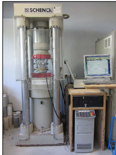
Figure 2-32 : Essai de compression simple
