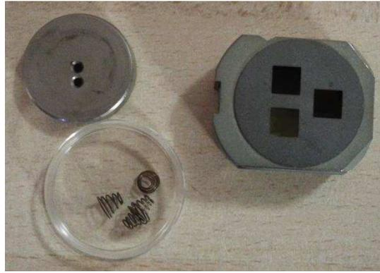
Fig.2. 2: Example of typical sample holder of 1 inch diameter for Cameca IMS5f SIMS equipment
