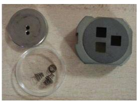
Fig.2. 2: Example of typical sample holder of 1 inch diameter for Cameca IMS5f SIMS equipment
