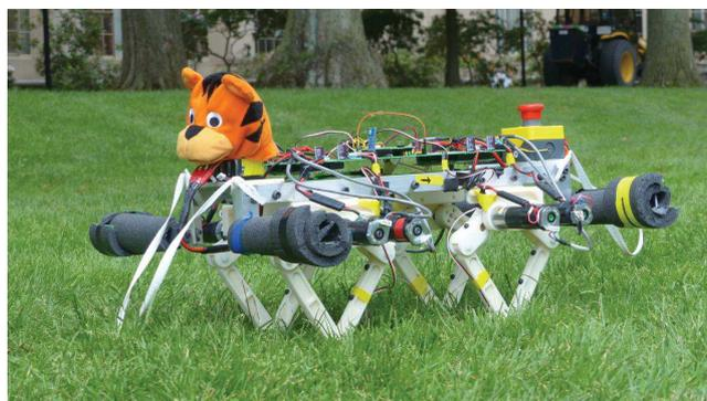
FIGURE 1.2 – Robot Super Mini Cheetah inspiré du guépard (source : <http://biomimetics.mit.edu/research/mit-super-mini-cheetah>)
