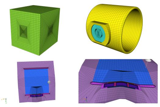
Figure 9.1.1 – The mesh LMJ, which is our industrial test case. Top left: the whole domain, which is in a cube. Top right: the capsule that is inside the cube. Bottom left: upper view of the interior of the capsule. The interior is colored in blue, cells containing gold are in pink, cells containing foam are in purple. Bottom right: side view of the capsule. Red cells are the slits in the foam.
