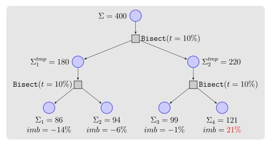
The heaviest part,  $\Pi_4$ , reaches a weight of  $\Sigma_4 = 121$ , which accounts for an imbalance of  $imb = \frac{\Sigma_4 - \frac{\Sigma}{k}}{\frac{\Sigma}{k}} = \frac{121-100}{100} = 21\%$ . Thus, the final imbalance of the partition far exceeds the input tolerance of 10%.
