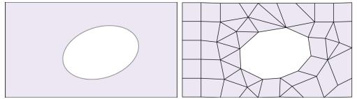
(a) A 2D bounded domain  $\Omega$  in 2D-(b) A mesh discretizing  $\Omega$  using triangles space and quadrilaterals
