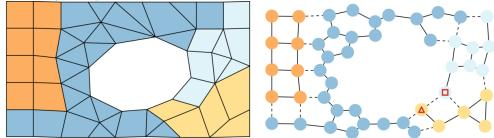
Figure 2.4.2 – 4-partition of a mesh and of its corresponding graph
