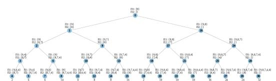
Figure 3.2.2 – The complete greedy bipartitioning algorithm tree applied to the example set  $S_e = \{9, 8, 7, 4, 4\}$ . The leaves are all the partitions of  $S_e$ . Their absolute differences are indicated below. The node numbers correspond to the order in which they are visited. In this example, the optimal (and perfect) partition is obtained at node 11. Note that only half of the tree is shown, the other half being symmetric (but with number 9 in  $\Pi_2$ ).
