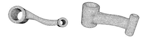
Figure 9.1.3 – Two different views of the 3D mesh Linkrodsok1, of 174218 cells
