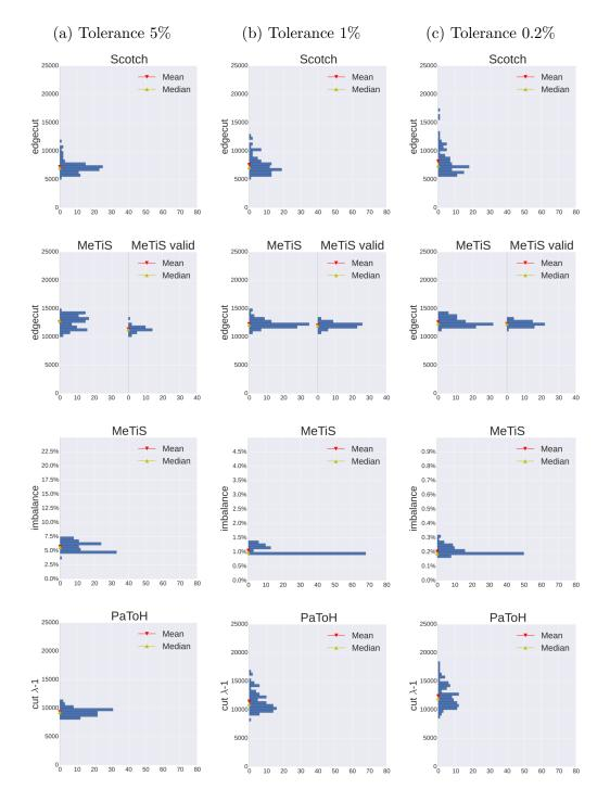
Figure 9.2.1 – Bar plots of the *edgecut*,  $cut_{\lambda-1}$  and *imbalance* of the partitions returned by Scotch, MeTiS and PaToH over 100 runs on the mesh *Mushroom*
