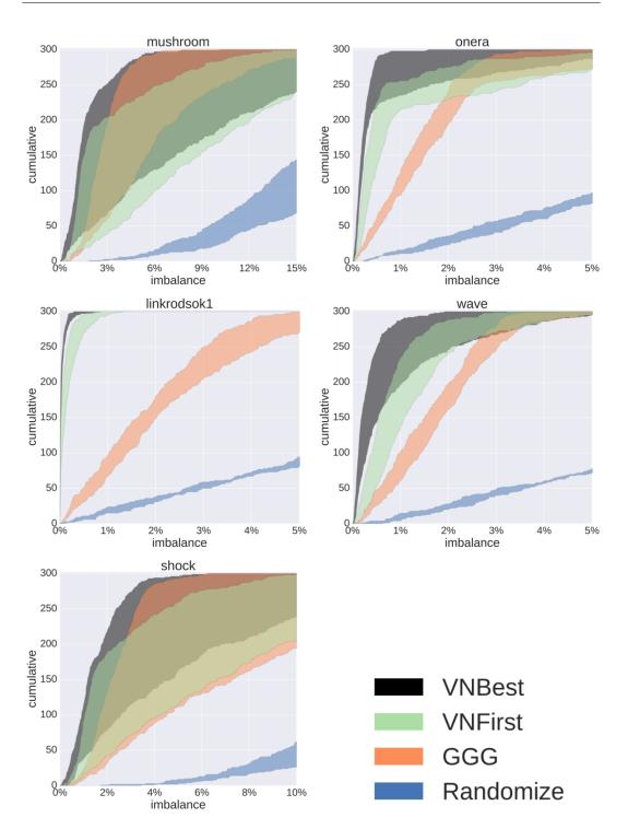
Figure A.3.1 – For a given algorithm, the *cumul* function introduced in Section 9.3.3 counts, given an imbalance x, the number of times that the algorithm returned a partition of imbalance smaller than or equal to x (therefore, left is better). The figure represents the area in which lies the *cumul* function of each initial partitioning algorithm, when partitioning the coarsest graph produced by different **Restriction** policies.
