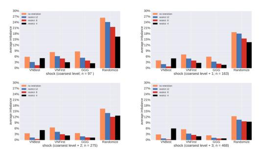
Figure A.3.7 – Average of the imbalance of the partitions returned for the mesh Shock at different coarse levels. The average was computed over 100 runs on each of the three weight distributions.
