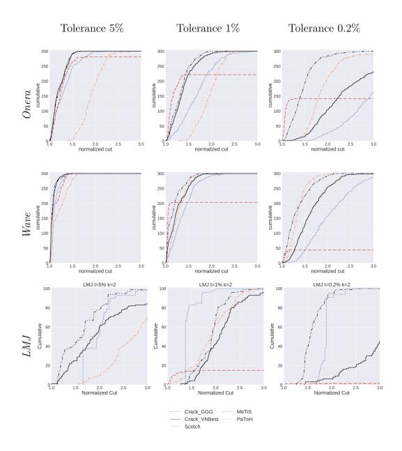
Figure 10.2.2 – Comparison of Crack, Scotch, MeTiS and PaToH on the three meshes, using the *cumul* function. For a given algorithm, cumul(x) is the number of solutions of communication cost smaller than x returned by the algorithm. Since we aim at minimizing the communication cost, top left is better.
