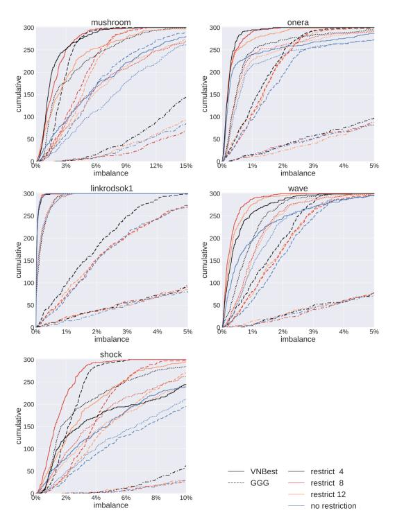
Figure A.3.2 – For a given algorithm, the *cumul* function introduced in Section 9.3.3 counts, given an imbalance x, the number of times that the algorithm returned a partition of imbalance smaller than or equal to x (Therefore, left is better). Dash types indicate the initial partitioning algorithm used, and colors indicate the **Restriction** policy.
