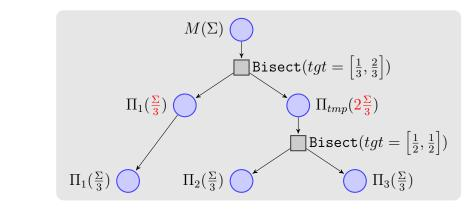
First, **Bisect** is applied on M, targeting a weight of  $\frac{\Sigma}{3}$  for part  $\Pi_1$  and  $\frac{2\Sigma}{3}$  for part  $\Pi_{tmp}$ . Then, **Bisect** is called on  $\Pi_{tmp}$  with "regular" target part weights, which means half the weight of  $\Pi_{tmp}$  for both parts. This forms  $\Pi_2$  and  $\Pi_3$ , both of weight  $\frac{2\frac{\Sigma}{3}}{2} = \frac{\Sigma}{3}$ .
