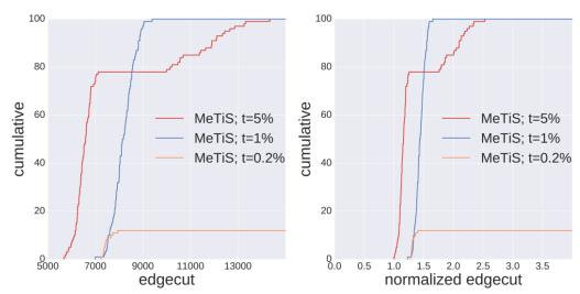
Figure 9.3.1 – *cumul* function for MeTiS on the mesh *Linkrodsok1*, for the first weight distribution. cumul(x) is the number of times that MeTiS returned a partition whose edgecut was smaller than x. Unlike on the left, the *edgecut* on the right plot is normalized with the minimal communication cost found by  $metis_5$ ,  $metis_1$  and  $metis_{0.2}$ , respectively.
