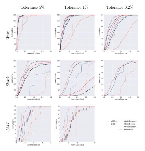
Figure 10.3.1 – Comparison of using different ordering policies on the communication cost of the partitions for three meshes, using the *cumul* function. For a given algorithm, cumul(x) is the number of solutions of communication cost smaller than x returned by the algorithm. Since we aim at minimizing the communication cost, top left is better.
