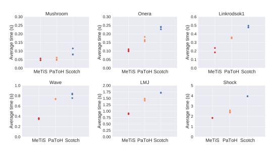
Figure 10.2.1 – Average time of Scotch, MeTiS and PaToH on each instance. Error bars are also displayed. For each algorithm, three points are plotted, corresponding to the imbalance tolerance of 5%, 1%, and 0.2%.
