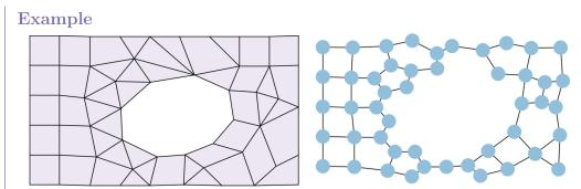
Figure 2.4.1 – Example of a mesh and its corresponding dual graph
