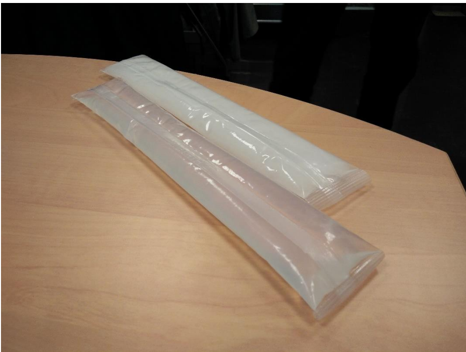
Annex A. 2 - Comparison between a two sticks with PCM in solid and liquid phase.
