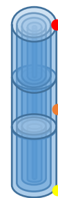
Figure 5. 12 - Position of the temperature sensors in relation to the discretization used for the modelling of a PCM stick.
