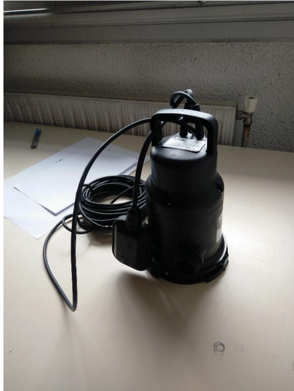
Annex A. 3 – Submersible pump
