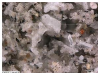
Fig. 1. Optical micrograph of a synthetic black crust before irradiation.
