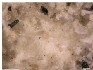
Fig. 2. Optical micrograph of a synthetic black crust after irradiation.
