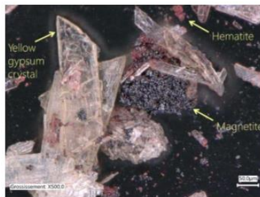
Figure 3 : Ejected particles collected on a glass slide (digital microscope picture)
