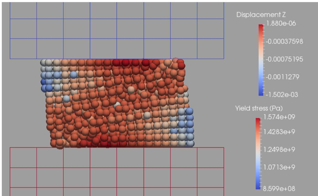
**Figure 3.19:** Final yield stress field without the J-C failure model
