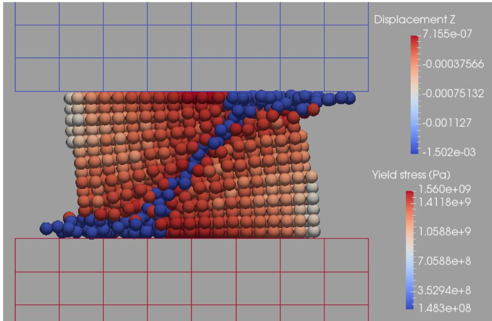
**Figure 3.35:** Yield stress field at final time in the case of a Shear failure criterion
