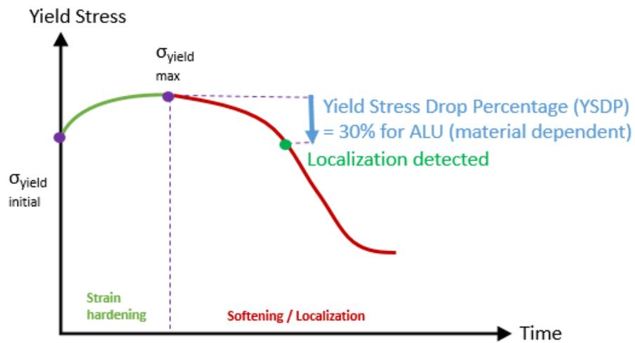
**Figure 2.3:** Schematic of the localization detection process
