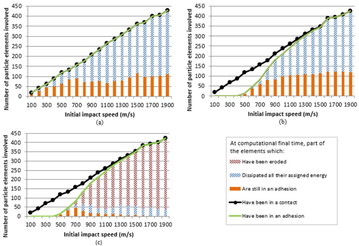
**Figure 3.48:** Behavior of the model as a function of initial particle speed, without criteria (a), with adhesion initiation criterion (b), and with adhesion initiation and erosion criteria (c), for the test case of Al/Al full SPH model
