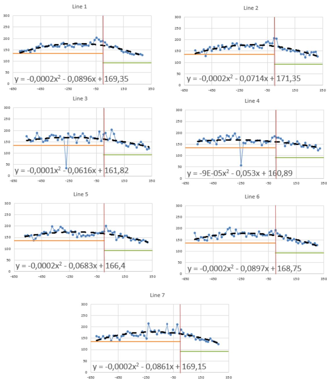
Vickers hardness variation for each indentation line on the  $230 \text{ m.s}^{-1}$  sample, as a function of distance to the interface (in microns).
