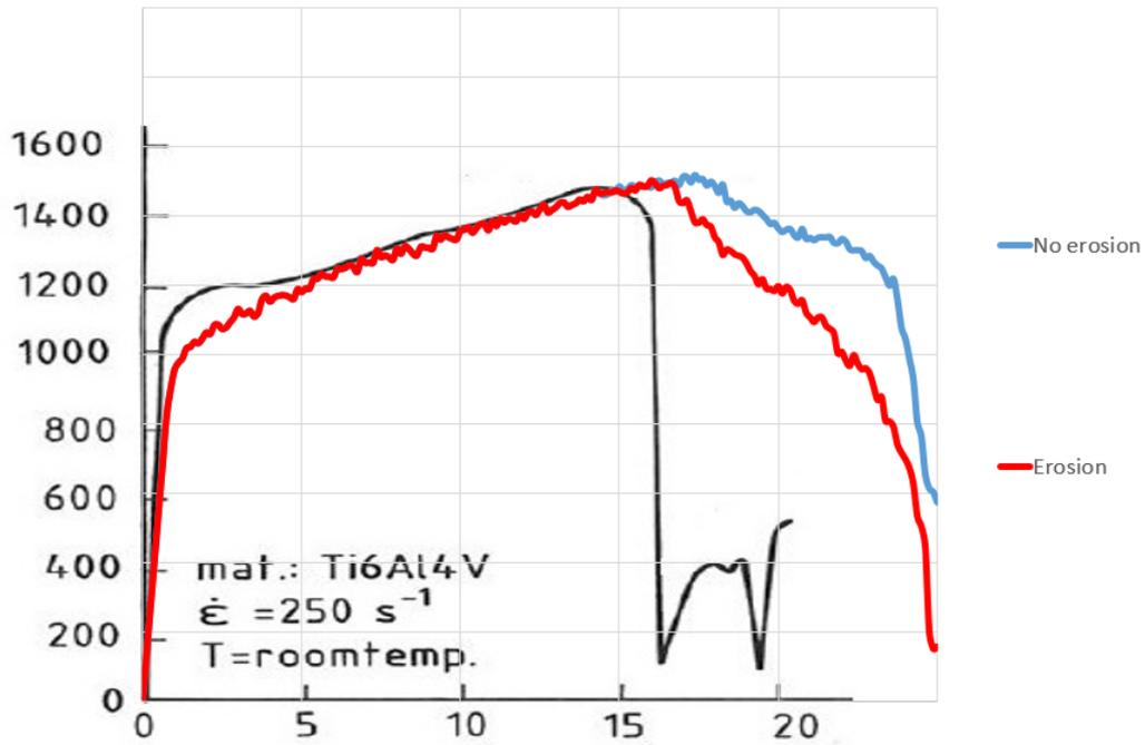
Figure 3.27: Effect of erosion on the response of the tilted cylinder
