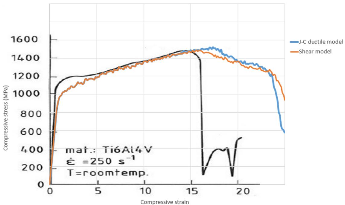
**Figure 3.32:** Stress-strain curve for the Shear failure model
