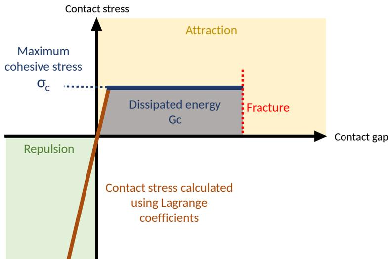
**Figure 2.2:** Schematic of the adhesive interaction law
