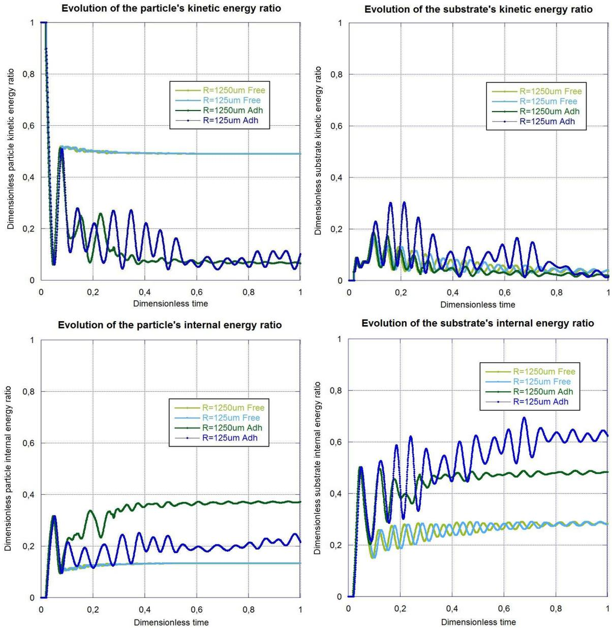
**Figure 3.42:** Energy distribution during the cylinder impacts
