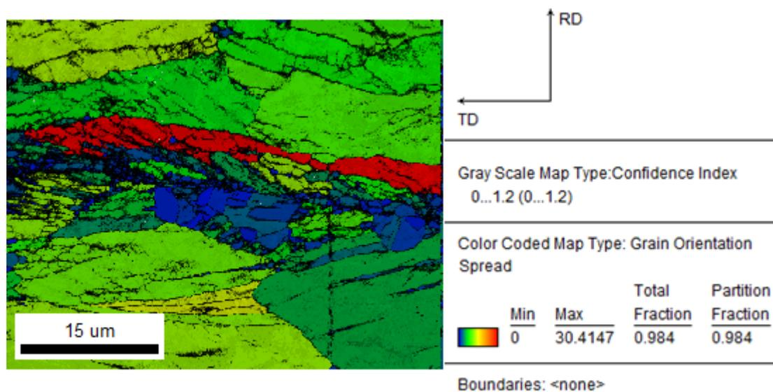
**Figure 4.31:** Grain Orientation Spread of the sample of impact speed  $230 \text{ m.s}^{-1}$
