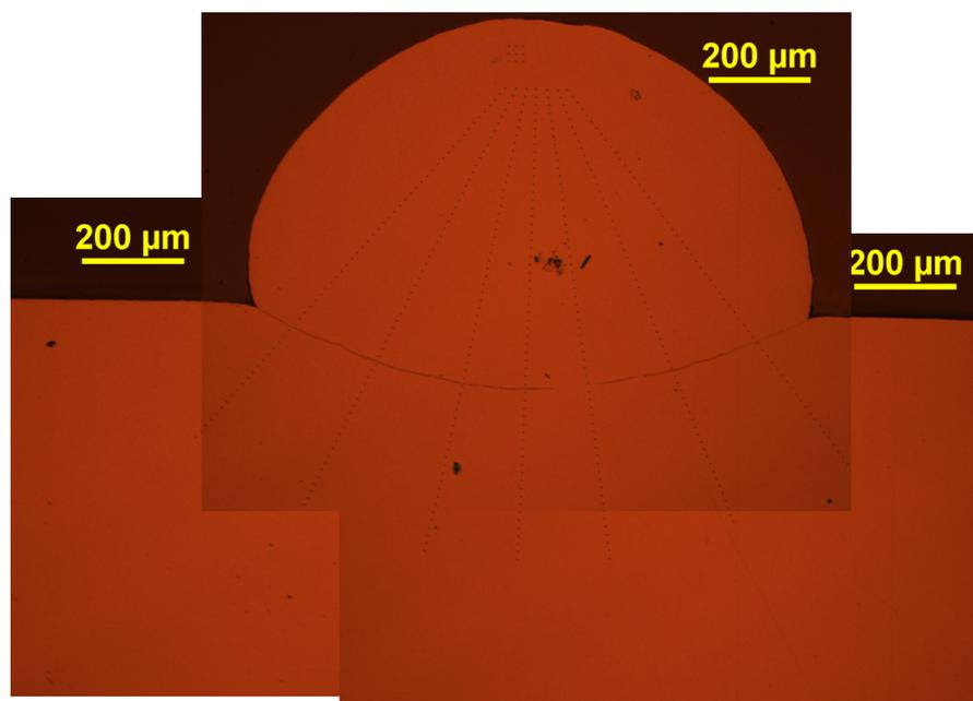
**Figure 4.56:** Cross-section view of the copper on copper SPSS impact at  $230 \text{ m}\cdot\text{s}^{-1}$
