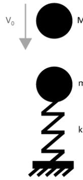
**Figure 3.39:** The basic impact model
