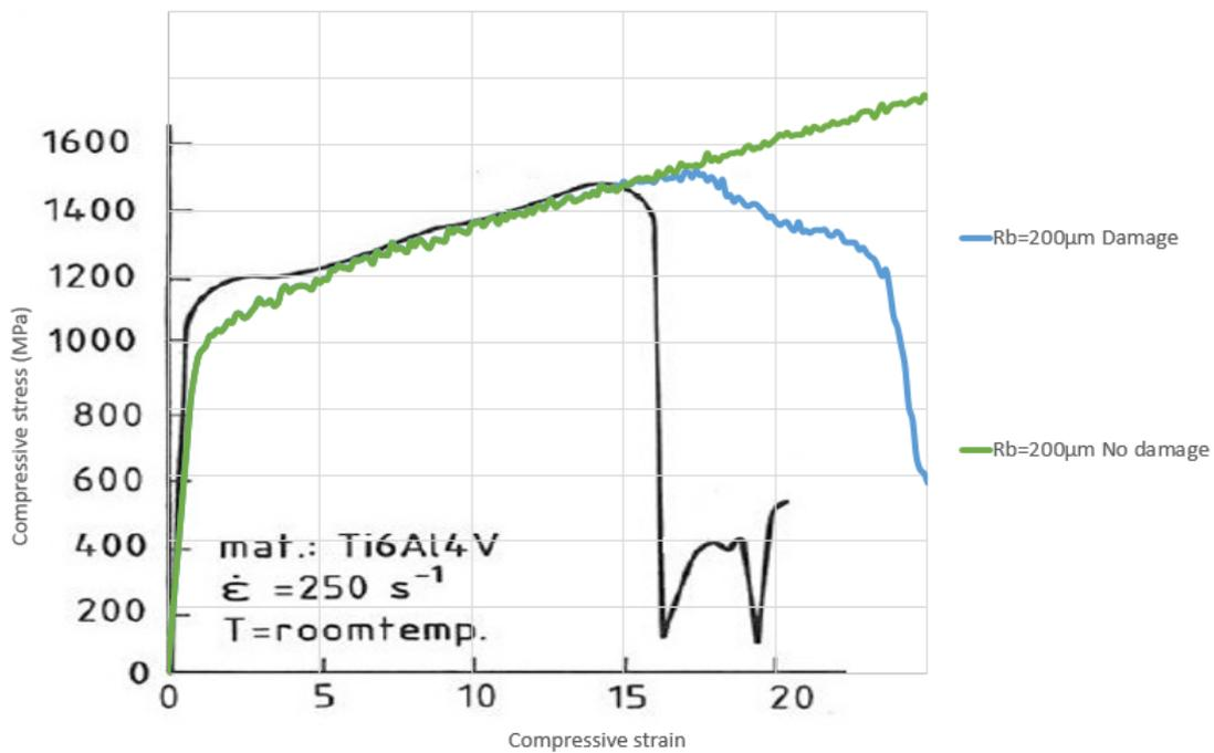
**Figure 3.18:** Effect of the J-C failure model on the localization in the Shear Banding model
