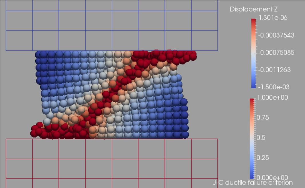
Figure 3.22: J-C failure criterion field, activating damage
