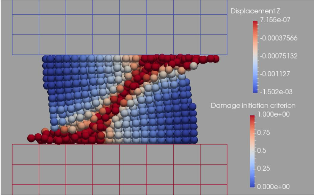
Figure 3.33: Damage initiation criterion field at final time in the case of a Shear failure criterion
