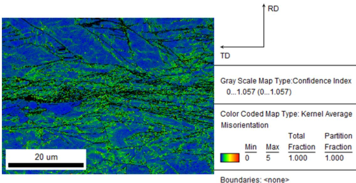
**Figure 4.27:** Kernel Average Misorientation of the sample of impact speed  $230 \text{ m.s}^{-1}$
