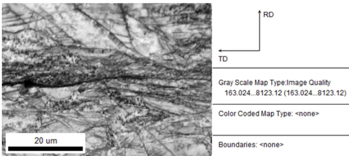
**Figure 4.26:** Image Quality of the sample of impact speed  $230 \text{ m.s}^{-1}$
