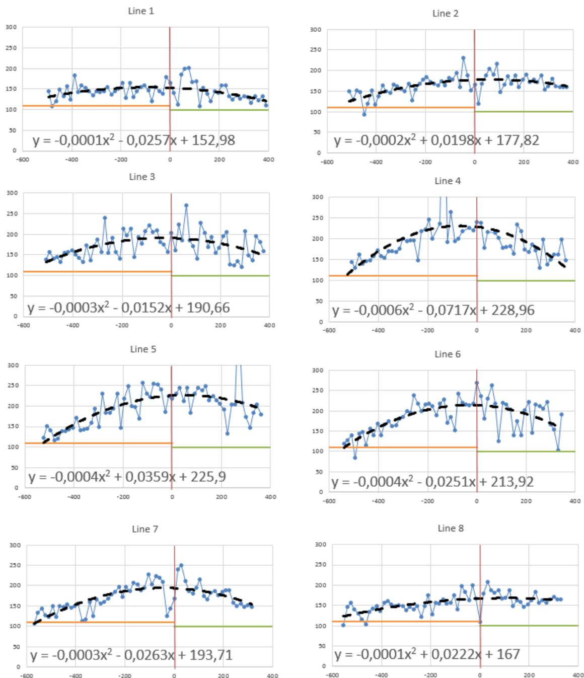
Vickers hardness variation for each indentation line on the  $457 \text{ m.s}^{-1}$  sample, as a function of distance to the interface (in microns).
