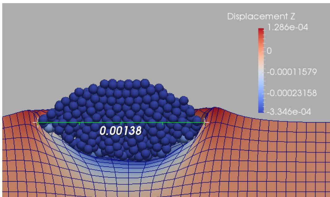
**Figure 4.57:** Cut view of the simulated copper on copper SPSS impact at  $457 \text{ m} \cdot \text{s}^{-1}$  with vertical displacements
