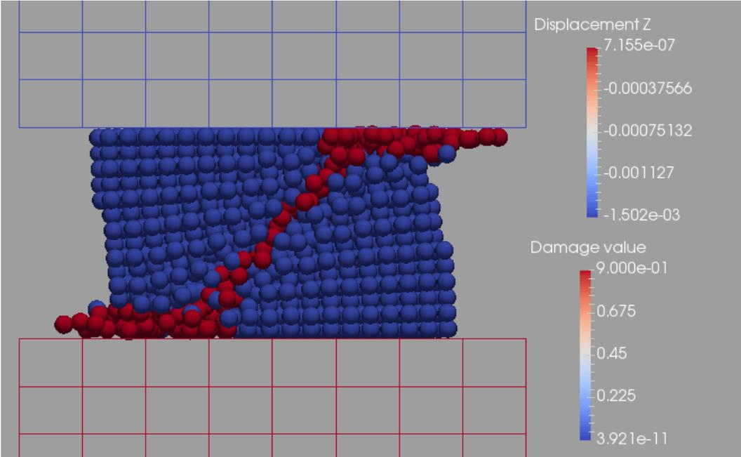
Figure 3.34: Damage field at final time in the case of a Shear failure criterion
