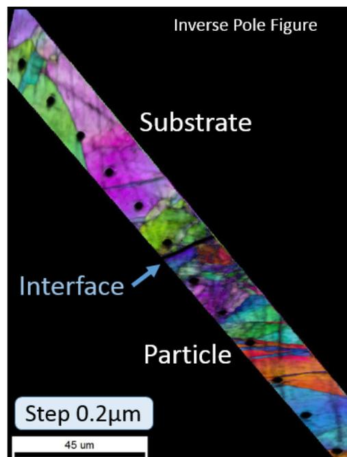
**Figure 4.47:** Example of Inverse Pole Figure of a zoom on indentations used for grain size measurement of the sample impacted at  $230 \text{ m.s}^{-1}$
