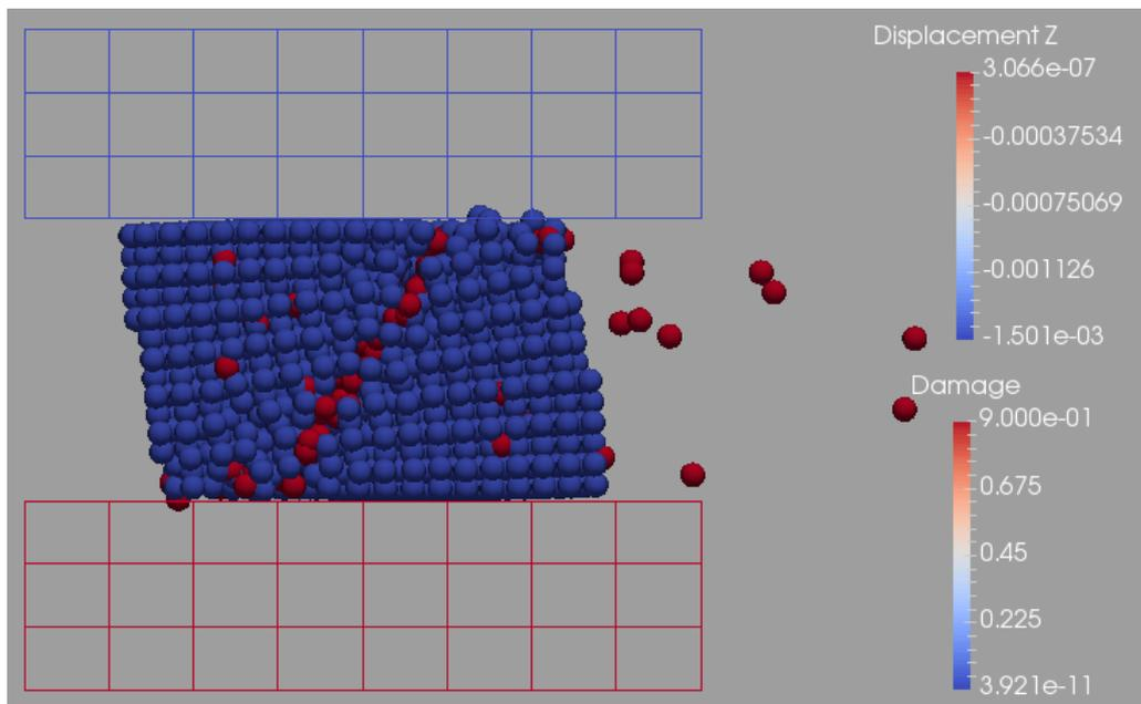
Figure 3.28: Damage field at final time in the case of erosion
