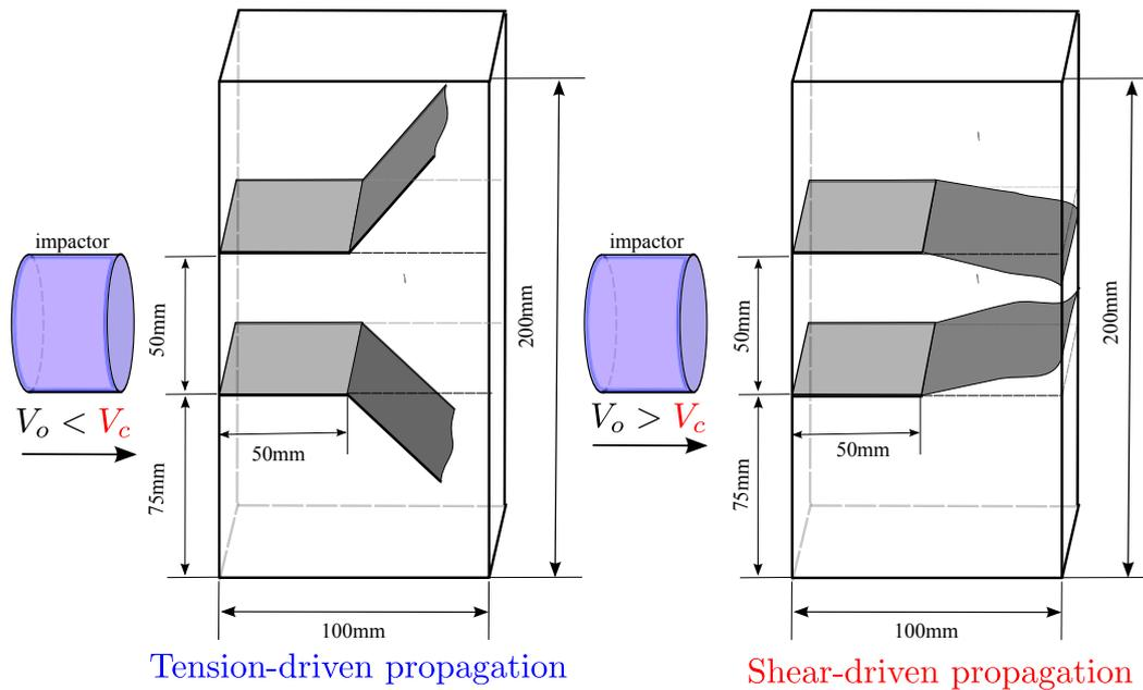
**Figure 1.4:** Kalthoff fast impact experiment [KAL 87]
