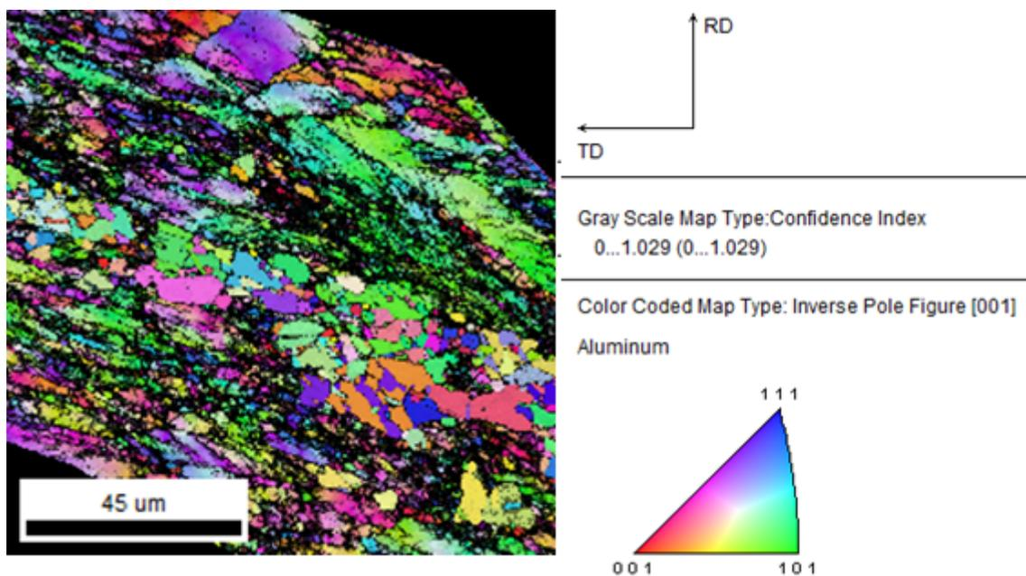
Figure 4.41: Inverse Pole Figure of the sample of impact speed  $457 \text{ m.s}^{-1}$
