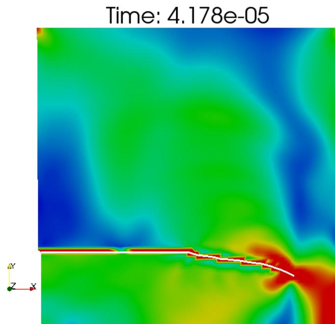
**Figure 1.5:** Shear bands formation for 32.41 m/s velocity [HAB 12]
