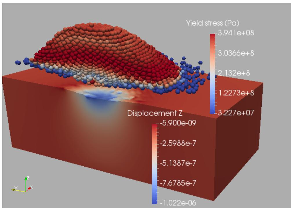
**Figure 3.37:** Yield stress field at final time in the case of 25 μm SPH copper particle impacting an FE aluminum substrate at 500 m.s<sup>-1</sup>
