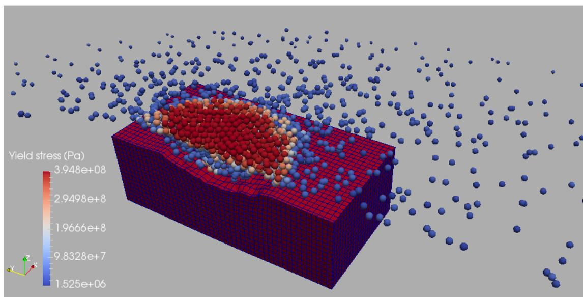
**Figure 3.38:** Yield stress field at final time in the case of 25 μm SPH copper particle impacting an FE aluminum substrate at 900 m.s<sup>-1</sup>
