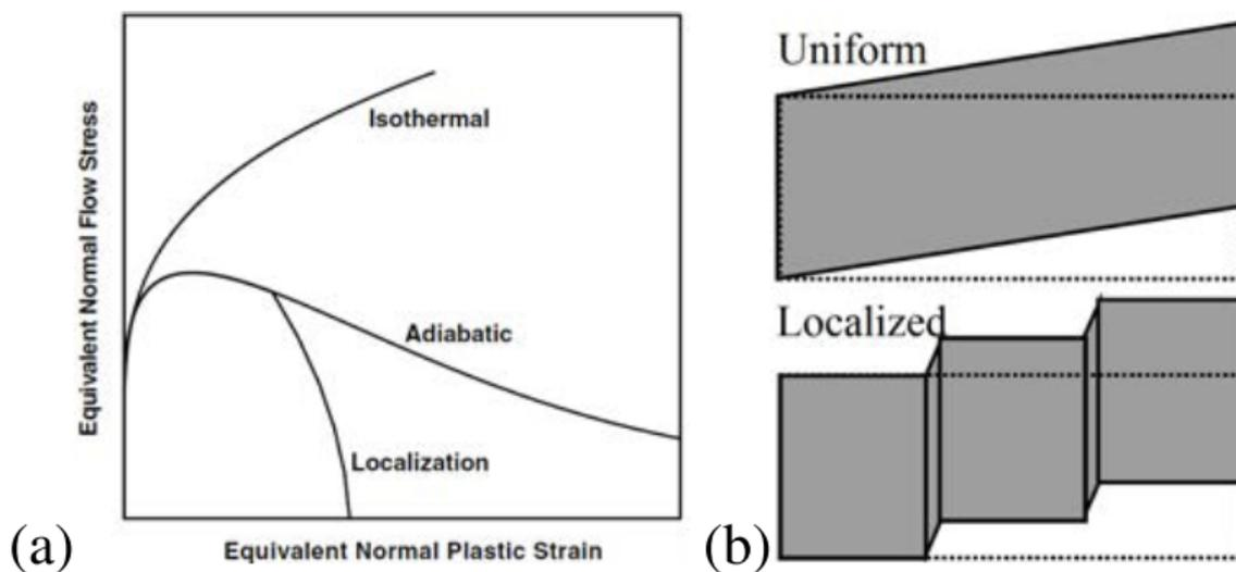
**Figure 1.6:** (a) Typical stress-strain curves in a normal strain hardening material (Isothermal), an adiabatically softened material (Adiabatic) and in a material undergoing an adiabatic shear localization (Localization); (b) schematics of the uniform and the localized simple shears [CHA 05].
