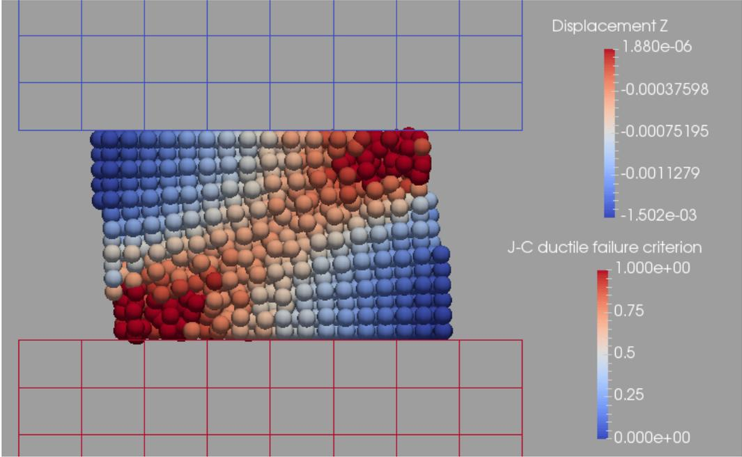
Figure 3.21: J-C failure criterion field, without activating damage
