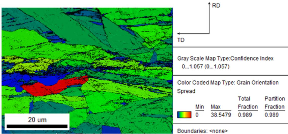
**Figure 4.28:** Grain Orientation Spread of the sample of impact speed  $230 \text{ m.s}^{-1}$
