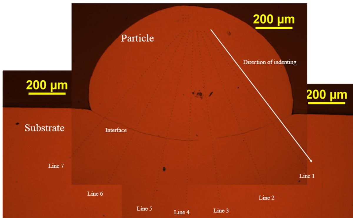
**Figure 4.1:** Indentations on the sample impacted at  $230 \text{ m.s}^{-1}$
