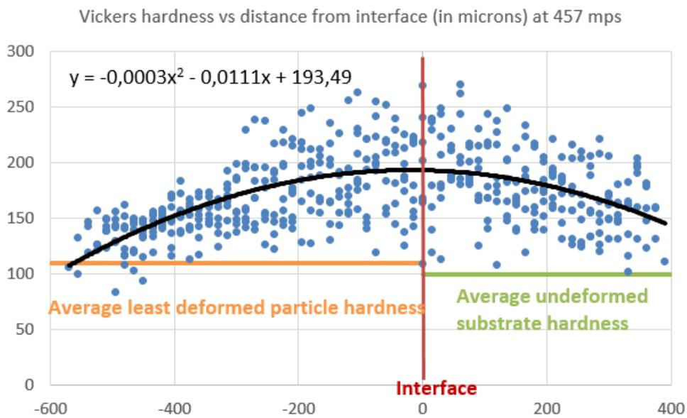
**Figure 4.5:** Hardness variations on the sample impacted at 457 m.s<sup>-1</sup>
