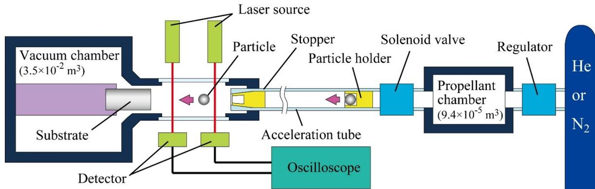
**Figure 1.10:** Diagram of the SPITS apparatus from [ITO 16]
