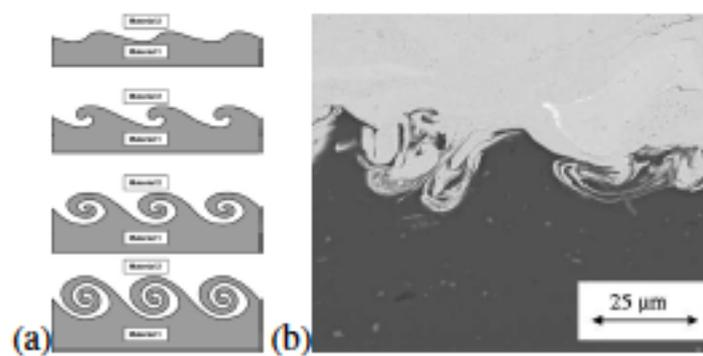
**Figure 1.8:** Material Mixing at interface [GRU 03, CHA 05]
