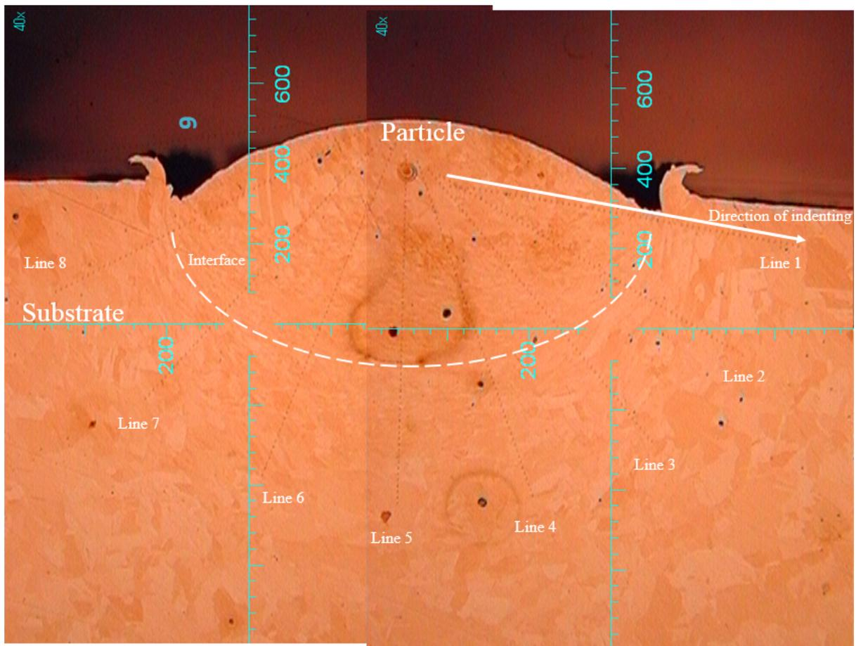
**Figure 4.4:** Indentations on the sample impacted at 457 m.s<sup>-1</sup>
