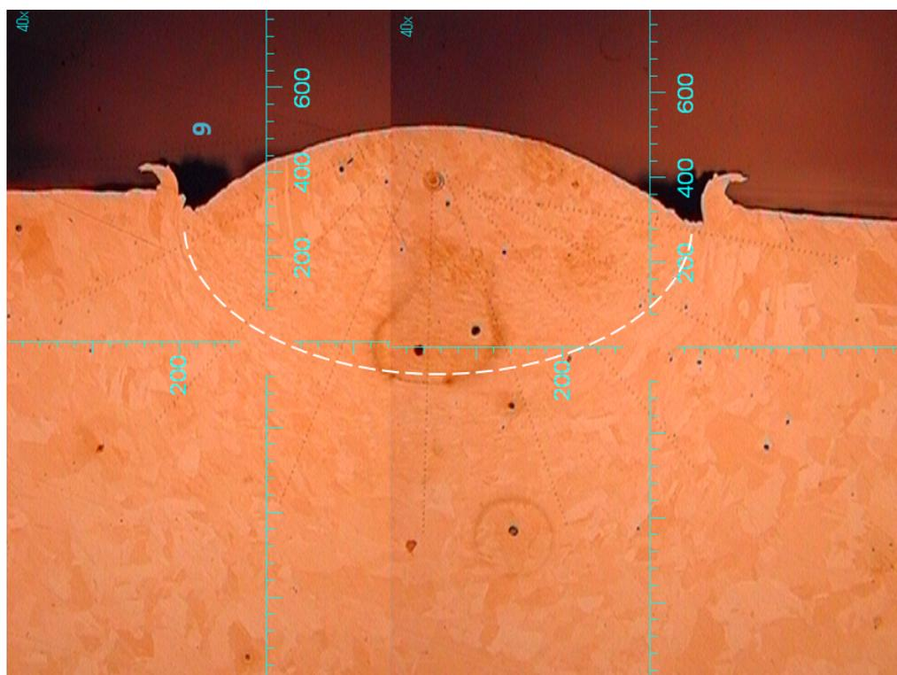
**Figure 4.58:** Cross-section view of the copper on copper SPSS impact at  $457 \text{ m} \cdot \text{s}^{-1}$
