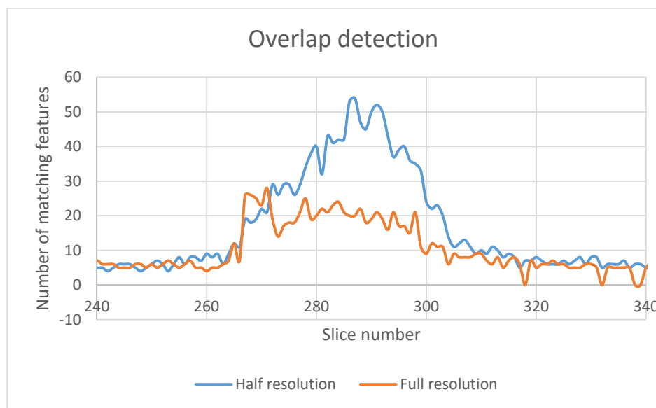
Figure 5.6. Overlap detection curve for the same set of Light Sheet Fluorescent Microscopy Acquisition images of Drosophila melanogaster brain of different resolutions: 0.177 \times 0.177 \times 0.469 \mu\text{m} (orange curve) and 0.354 \times 0.354 \times 0.469 \mu\text{m} (blue curve).
