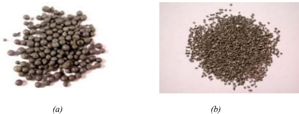
Figure 1.9 (a) Lead particles; (b) tungsten carbide particles [192].
