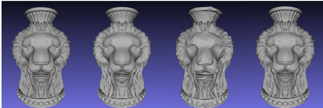
Figure 2.7: An example of different smoothing methods. From left to right: Original Vase Lion model with 38,728 points; Laplacian smoothing, iteration steps: 3; Two-step smoothing, iteration steps: 3, feature angle: 30 degree, normal smoothing steps 10, vertex fitting steps 10; Taubin smoothing, iteration steps: 3, \lambda = 0.5 , \mu = -0.53 . All the models are processed by the software Meshlab [19].
