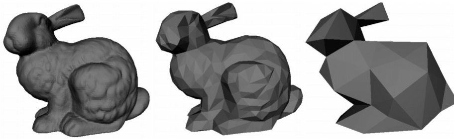
Figure 2.9: Different simplified Bunny models using quadric edge collapse decimation for different target triangles. From left to right: Original Bunny model with 69,451 triangles; A simplified Bunny model with 1,000 triangles; A simplified Bunny model with 100 triangles. The image is from [37].
