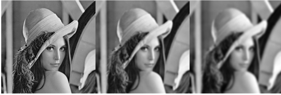
Figure 2.3: A smoothing example using Gaussian filter with different \sigma values. From left to right: Original Lena image, size: 512 \times 512 ; Image with Gaussian smoothing, \sigma=3 ; Image with Gaussian smoothing, \sigma=5 . The original image is manipulated by MATLAB .
