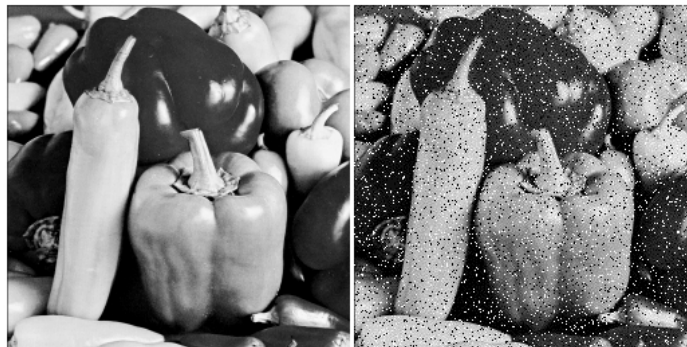
Figure 2.2: Left: Original Pepper image, size: 256 \times 256 , Right: Fat-tail distributed noise (added to 10% of the pixels). The noise is added by using MATLAB .
