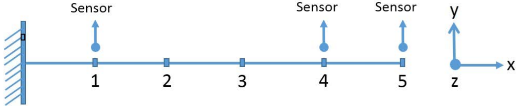
Figure 8.4 – 2D Beam model with 5 elements (15 DOFs) -using three sensors at nodes 1, 4, and 5 in y-direction
