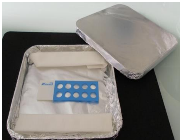
Fig. 1. Wet chamber (a square Petri dish containing wet filter paper to keep air humidity).
