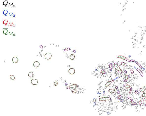
FIGURE 4.24: Comparison of the raw and filtered Q-criterion in a crossing plane
