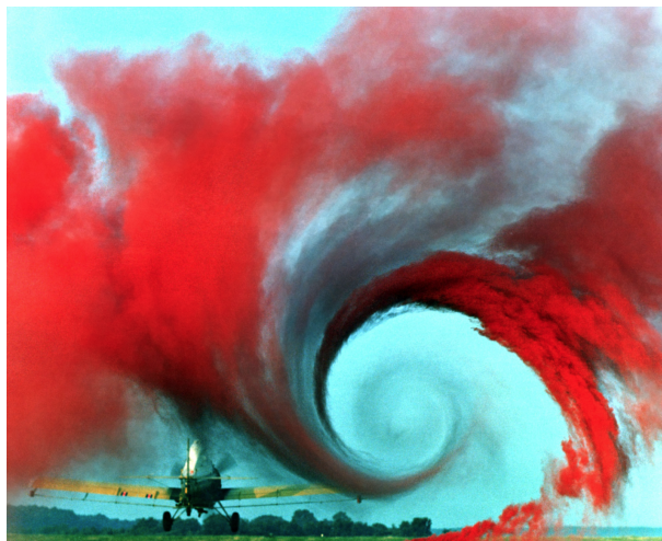
FIGURE 2.2: Vortices produced by plane take-off from [31]
