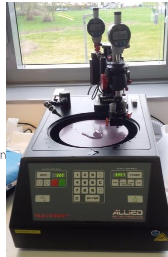
Figure 0.1: Schematic and the photograph of Chemical and Mechanical Polishing (CMP) process system that we used for thinning the silicon substrates.
