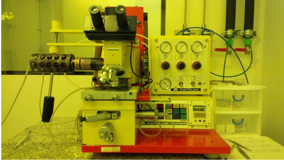
Figure 0.2: Photograph of the MJB3 Mask aligner for UV photolithography in cleanroom of class 1000 (ISO 6) at GREYC laboratory
