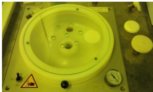
Figure 0.1: Photograph of spin coater used to apply photoresist on the surface of different materials such as LSMO, SOI, etc. in the cleanroom of class 1000 (ISO 6) at GREYC Laboratory.
