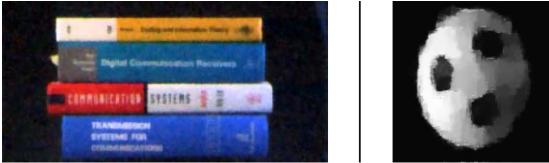
FIGURE I.7 – Lensless single-pixel camera images adapted from Huang et al. (2013) (left), and the single-pixel camera image obtained with a carbon nanotube photodetector adapted from Chen et al. (2014) (right).
