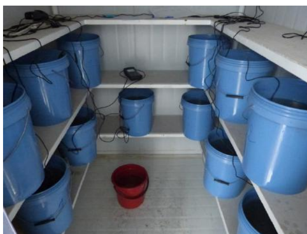
Image 4-1: Dark room used to incubate water samples during the decomposition experiment
