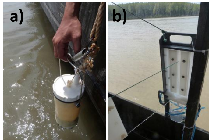
Image 3-1: a) Weighted bottle and b) glass plate sampler used for water layers sampling in the Can Gio mangrove estuary
