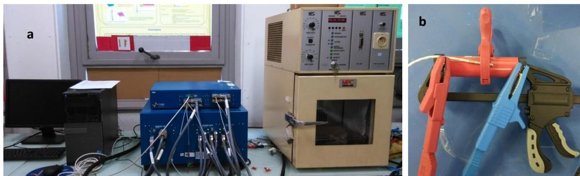
**Figure 2.1:** (a) Computer, potentiostat and the climatic chamber and (b) Connection's configuration of the Li-ion battery throughout the study.
