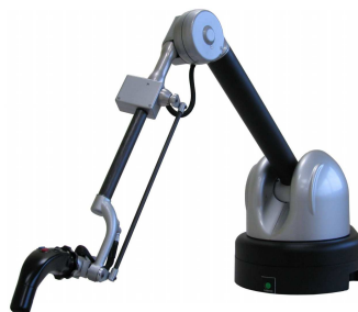
Figure 4.3: Virtuoso 6D (Haption S.A.). Haptic device used in this thesis work.
