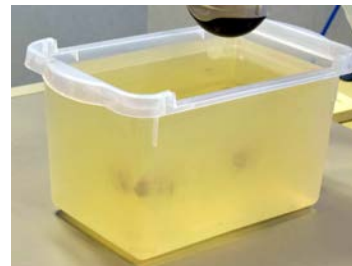
(b) Two-layers gelatin phantom containing two duck gizzards.
