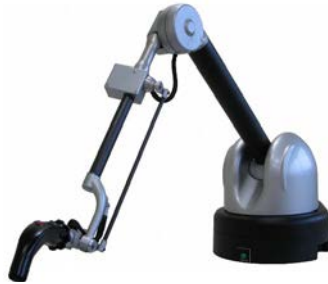
Figure 4.3: Virtuouse 6D (Haption S.A.). Haptic device used in this thesis work.
