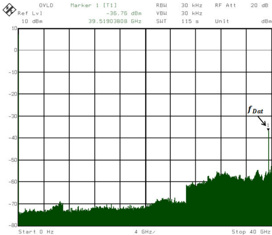
Figure 3.9: Electrical spectrum of the optical signal at the input port (C) at f_{Dat} = 39.5 GHz.
