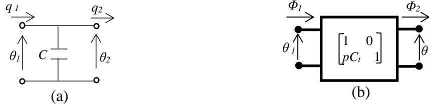
Fig. 4-12 Heat transfer model of a high conductivity medium: (a) network expression; (b) matrix expression.
