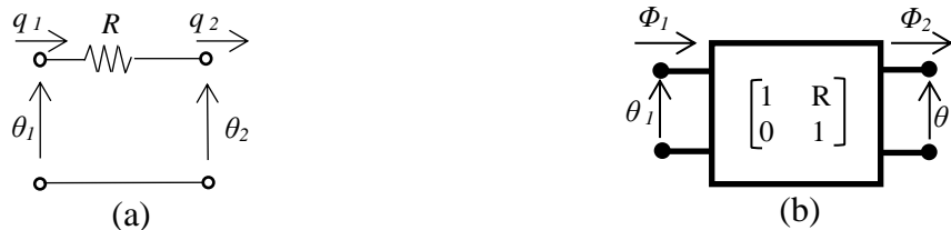
Fig. 4-11 Heat transfer model of a high resistance medium: (a) network expression; (b) matrix expression.
