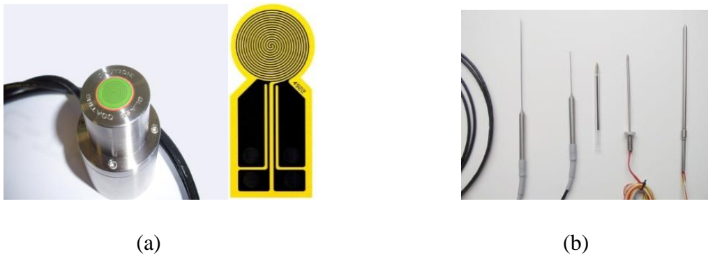
Fig. 1-7 (a) hot disc for transient plane source measurements (b) needle probe for transient line source measurements
