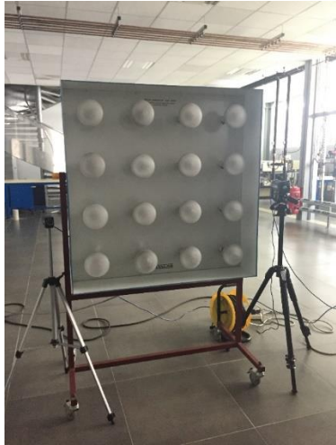
(a) artificial solar lamps and IR cameras
