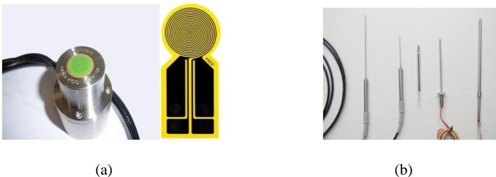
Fig. 1-7 (a) hot disc for transient plane source measurements (b) needle probe for transient line source measurements
