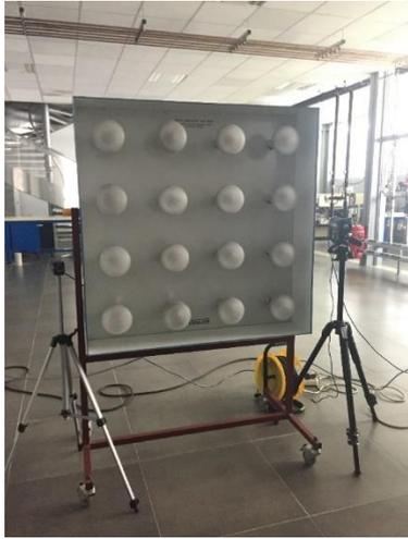
(a) artificial solar lamps and IR cameras
