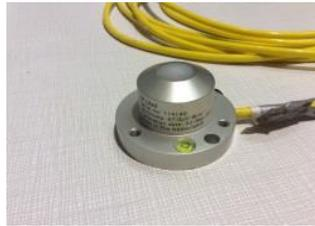
FIGURE 4 Silicon Pvrnometer for lambs calibration
