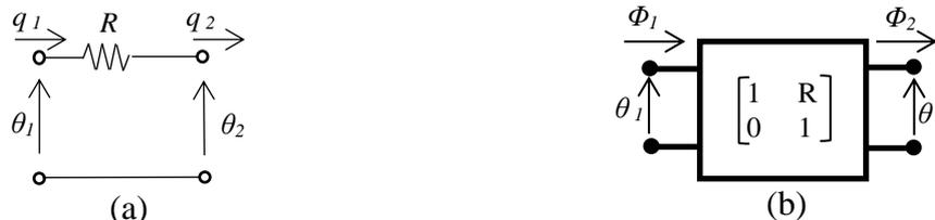
Fig. 4-11 Heat transfer model of a high resistance medium: (a) network expression; (b) matrix expression.
