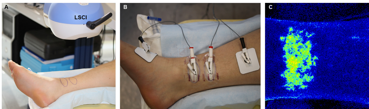
Fig. 1. Experimental setup. (A) Two ellipsoidal skin sites were chosen and marked on the ventral side of the right malleolus area. Microvascular blood flux was recorded using laser speckle contrast imaging. (B) Two iontophoresis electrodes connected to power supplies were placed on the right malleolus area according to the randomization assignment and 40 mC/cm 2 cathodal iontophoresis of treprostinil and placebo were performed. (C) Cutaneous perfusion recorded with LSCI at 1 h after treprostinil iontophoresis in a diabetic patient. Colors range from dark blue (no perfusion) to yellow and red (high perfusion). (For interpretation of the references to color in this figure legend, the reader is referred to the web version of this article.)
