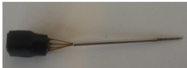
Figure 2.26. Picture of the single-unit microelectrodes used for in vivo acute electrophysiological recordings.
