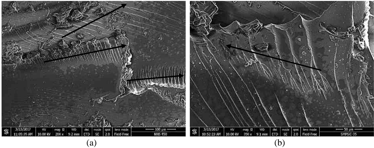
Figure 88 - SEM pictures of fracture profile of epoxy resin compressive samples (ET detector)
