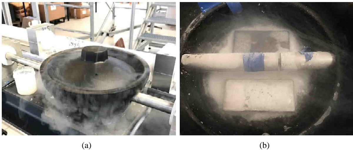
Figure 35 – Cryogenic system for SHPB setup (a) whole setup and (b) focus on the sample
