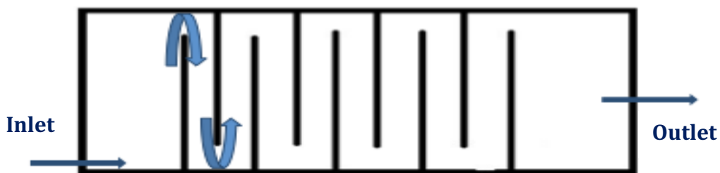
Figure 3. Scheme of the circulation of the microalgal suspension in the reactor. The black vertical segments represent the electrodes, and the arrows represent the zigzag path.
