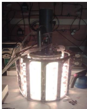
Figure 2. The photobioreactor used for Chlamydomonas reinhardtii culture.
