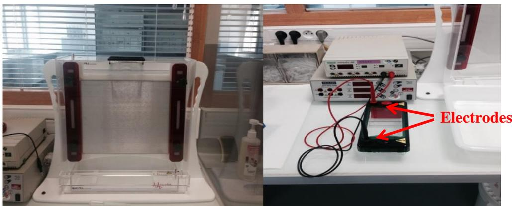
**Figure 2.10** The apparatus for polyacrylamide and agarose gel electrophoresis. The mold in which the gel was polymerized and stabilized was vertical for polyacrylamide gel (left) and horizontal for agarose gel (right). The electrodes in the apparatus could be connected to power supplier to apply electoral potential to the electrodes as shown in the figure.
