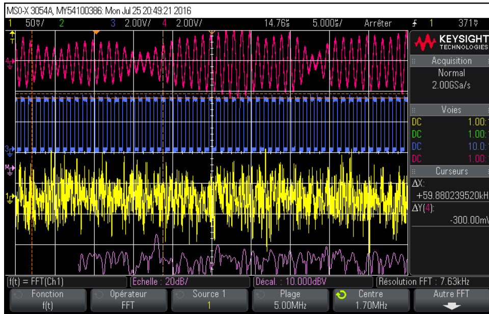
FIGURE 5.25: Illustration of the processing chain of the VLR: in yellow, input signal of peak-to-peak amplitude 20\text{ mV}_{pp} and \text{SNR} = 5\text{ dB} , in purple, its FFT, in pink, signal obtained after band-pass filtering and in blue square signal reconstructed by the high-speed comparator.
