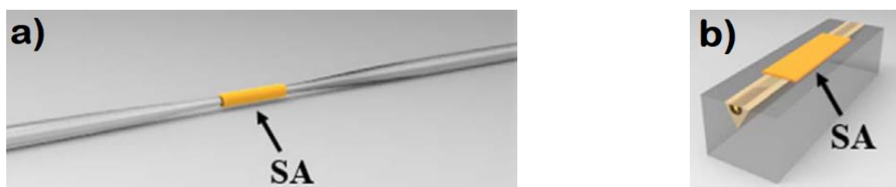
Figure 5:2. Saturable absorbers with evanescent field interaction: a) fiber taper (b) and side-polished (D-shaped) fiber.
