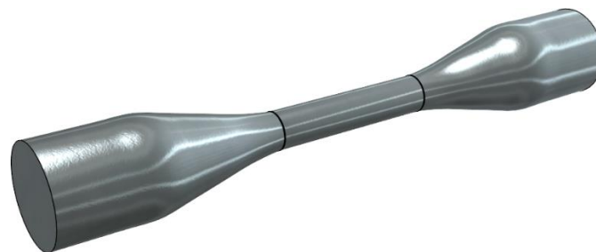
Figure 5:23. Microfiber optical taper schematic.
