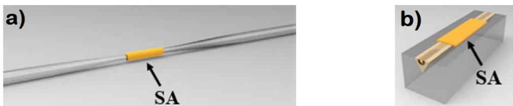
Figure 5:2. Saturable absorbers with evanescent field interaction: a) fiber taper (b) and side-polished (D-shaped) fiber.
