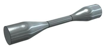
Figure 5:23. Microfiber optical taper schematic.
