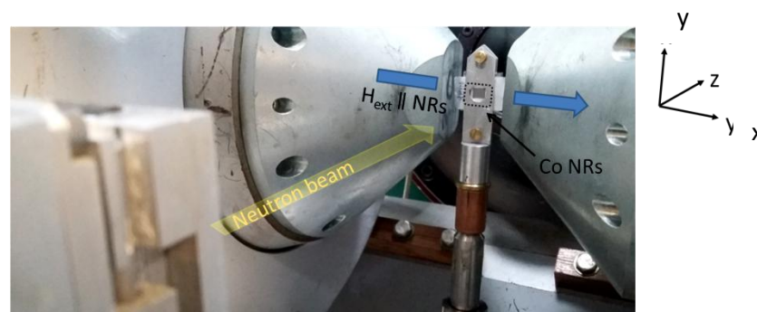
Figure IV- 13 Photograph of the experimental set-up showing the sample holder centered in between the coils of the electromagnet. The magnetic field was applied perpendicular to the neutron beam.
