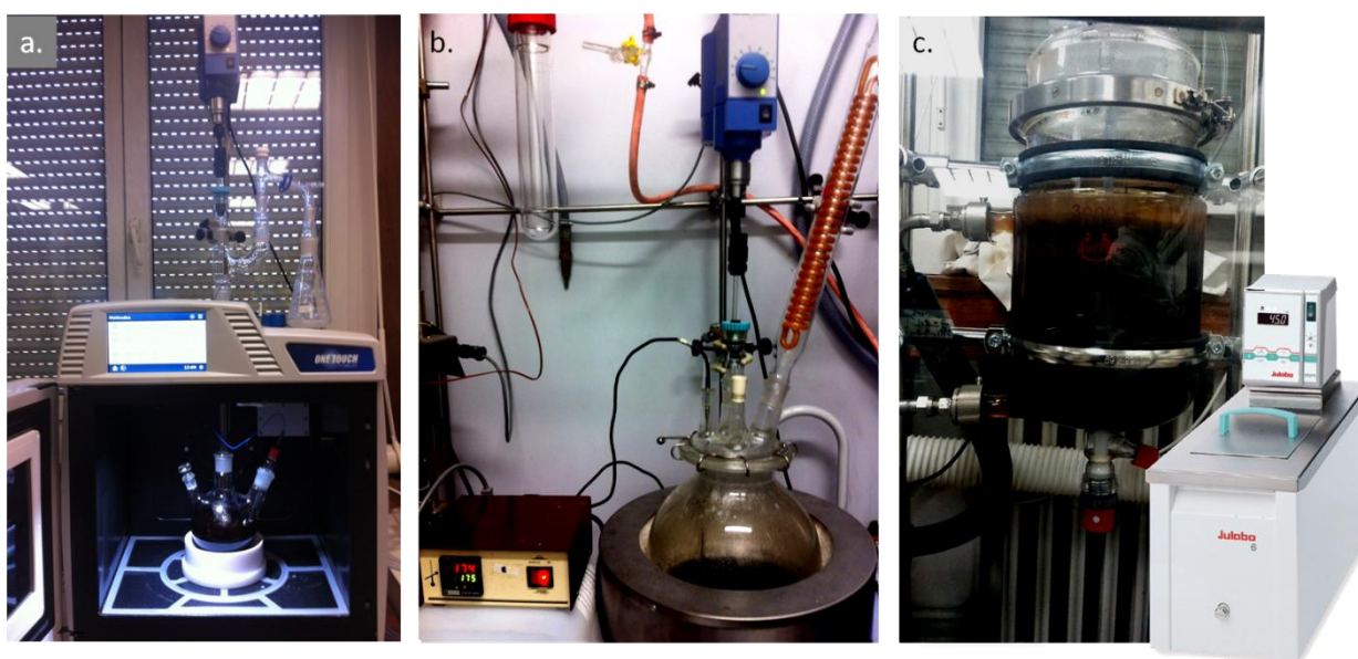
Figure II- 25 Heating set-ups: a. microwave; b. heating mantle; c. jacketed reactor.
