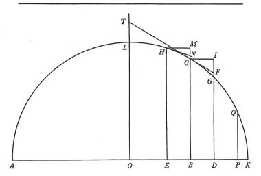
[8]<sup>(59)</sup> [Sit AK planum illud plano schematis perpendiculare, ALCK linea curva, C corpus in ipsa motum, et CF recta ipsam tangens in C. Fingatur corpus C progredi ab L ad K per lineam illam ACK, et interea impediri a Medio resistente. A puncto C ad rectam AK horizonti parallelam demittatur perpendiculum CB, et in recta illa sumantur hinc inde lineolæ æquales EB, BD,  $DP^{(60)}$  et
