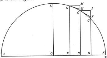
Sit AK planum illud plano schematis perpendiculare, ALCK linea curva, C corpus in ipsa motum, et CF recta ips[a]m tangens in C. Fingatur corpus C progredi ab L ad K per lineam illam ACK, et interea impediri a Medio resistente.
